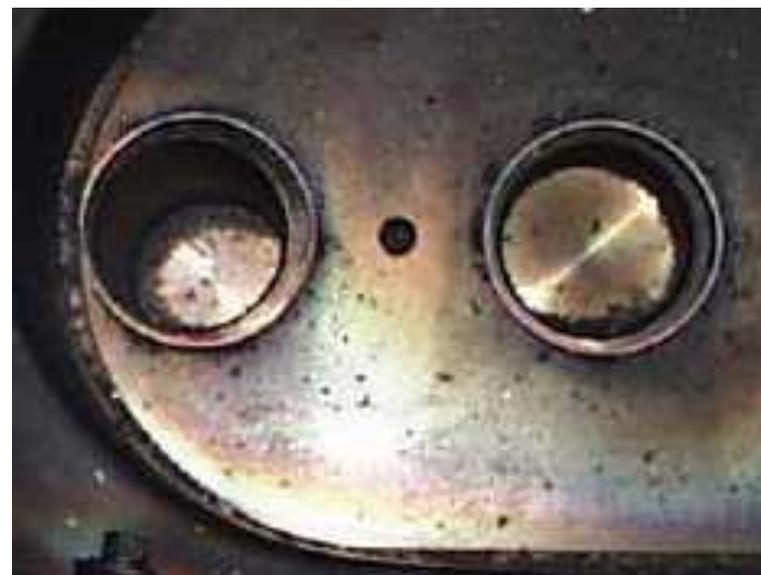
Debris and dust on TFTR vessel floor
