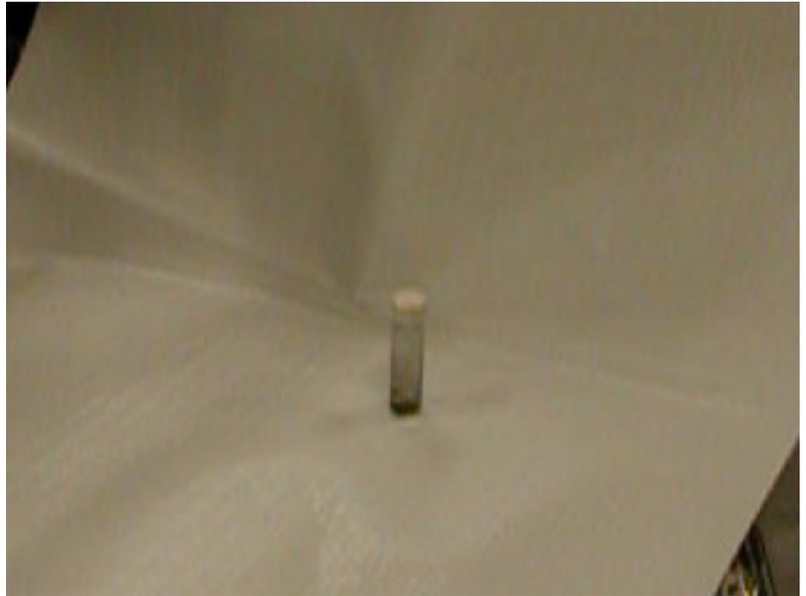
Samples of codeposit were scraped from TFTR tile KB3 for analysis. A small quantity was loaded into a small glass vial with a plastic cap for analysis of beta induced conductivity. In this process the plastic cap was rubbed by neoprene gloves.
