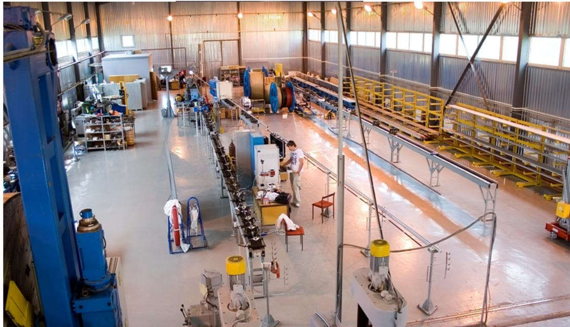
**The jacketing installation at Moscow's JSC VNIIEP Research Center where 760 metres of toroidal field dummy conductor were successfully produced in 2011.**
