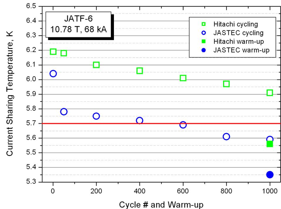
Cyclic loading tests have revealed problems...
