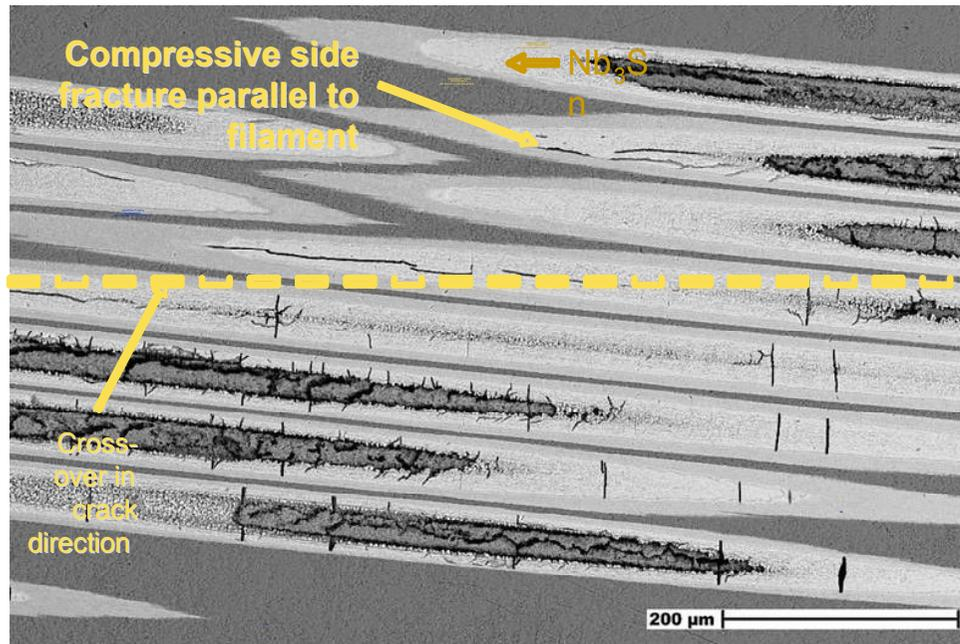
Longitudinal section of a bent strand, highlighting cracks in the tensile region.
