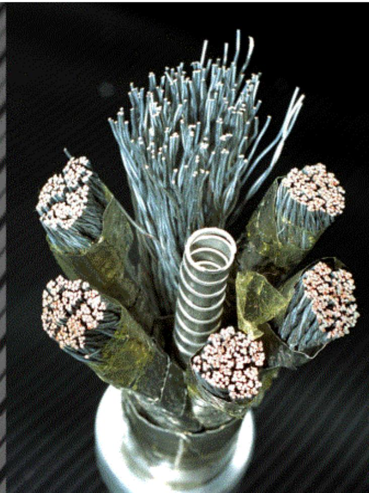
Superconducting cable for ITER
