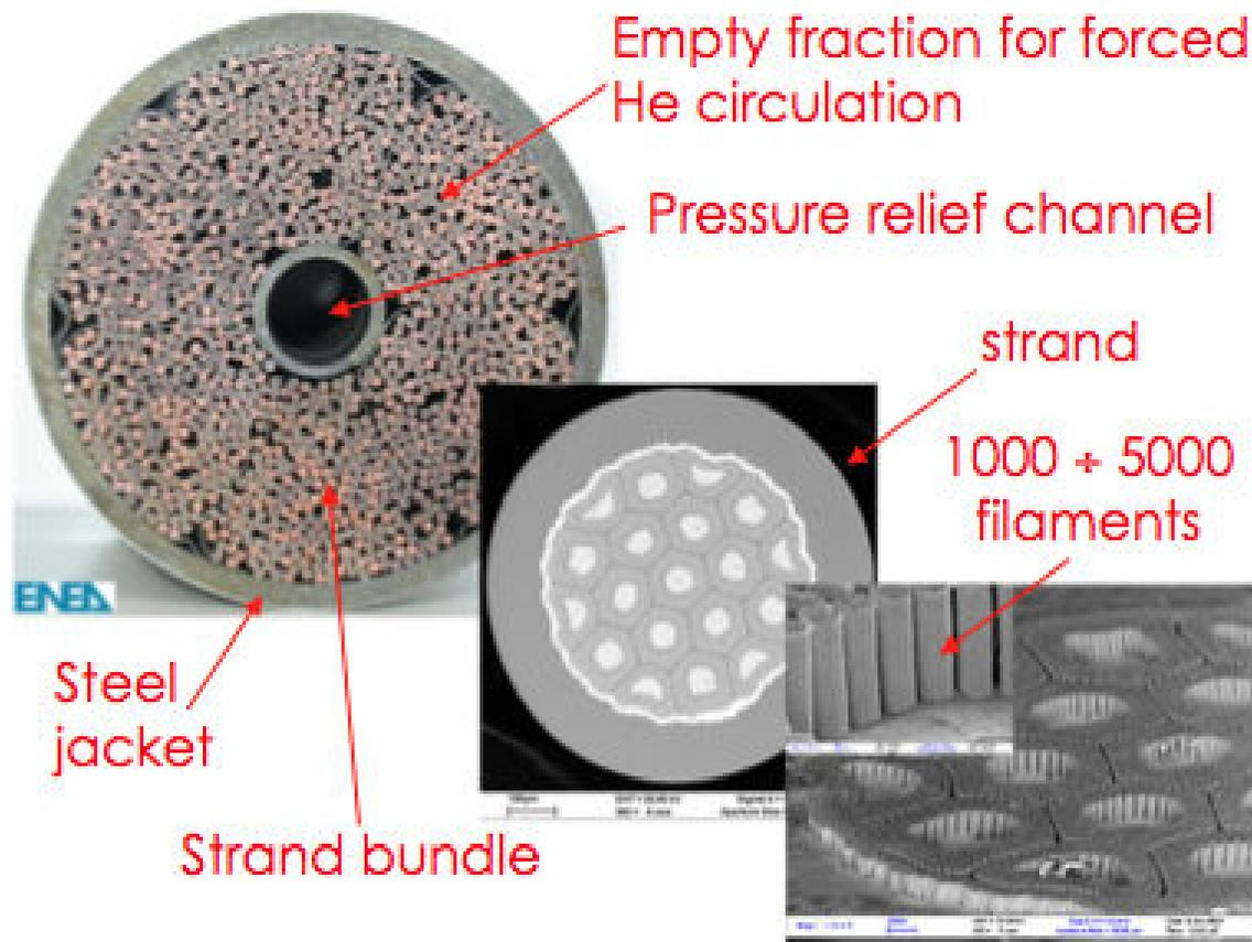
Typical construction of Cable in Conduit Conductor
