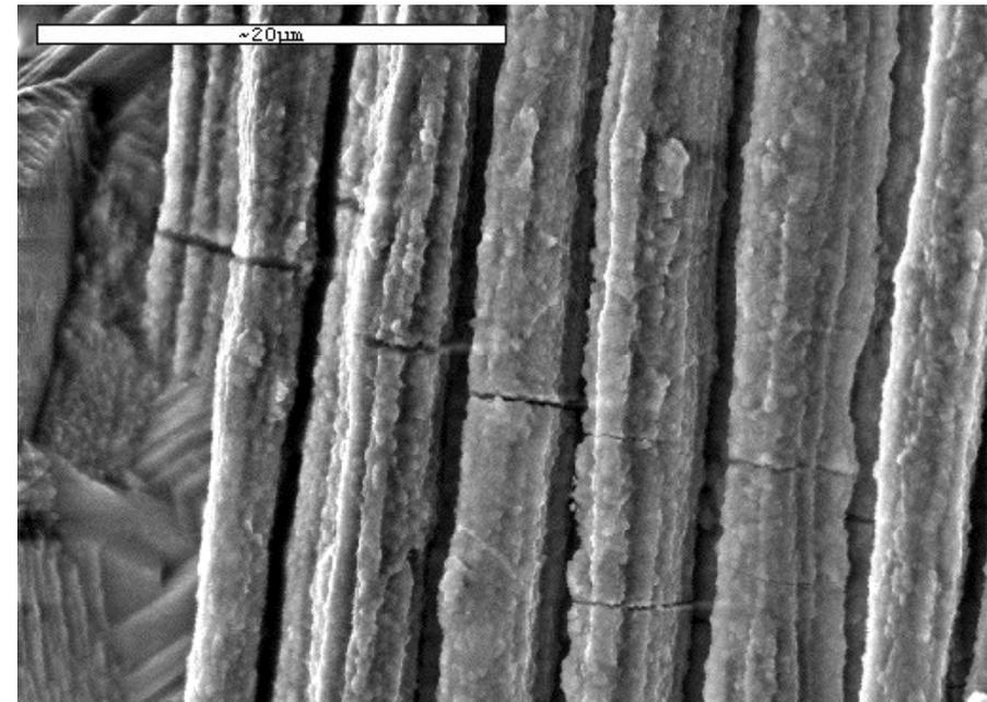
Scanning microscope image of etched filaments with crack propagation
