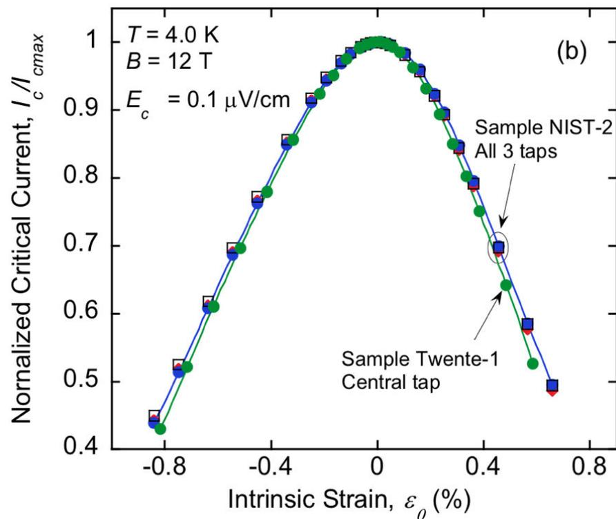
→ only about **50% ÷ 80%** of the current carrying capability of the material is actually available – **before any degradation**
