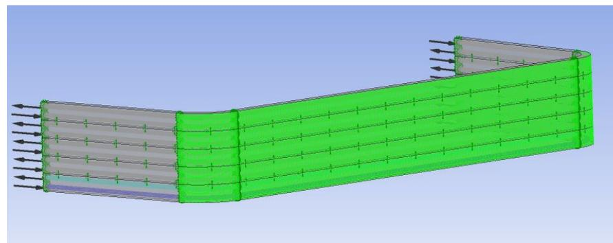
The ZV model had 5 pairs of cooling channels, the coolant flowing in the opposite direction in a pair.
