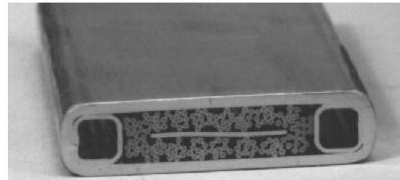
DPC-EX (2-stage flat cable, encased into a welded steel conduit and pipes)
