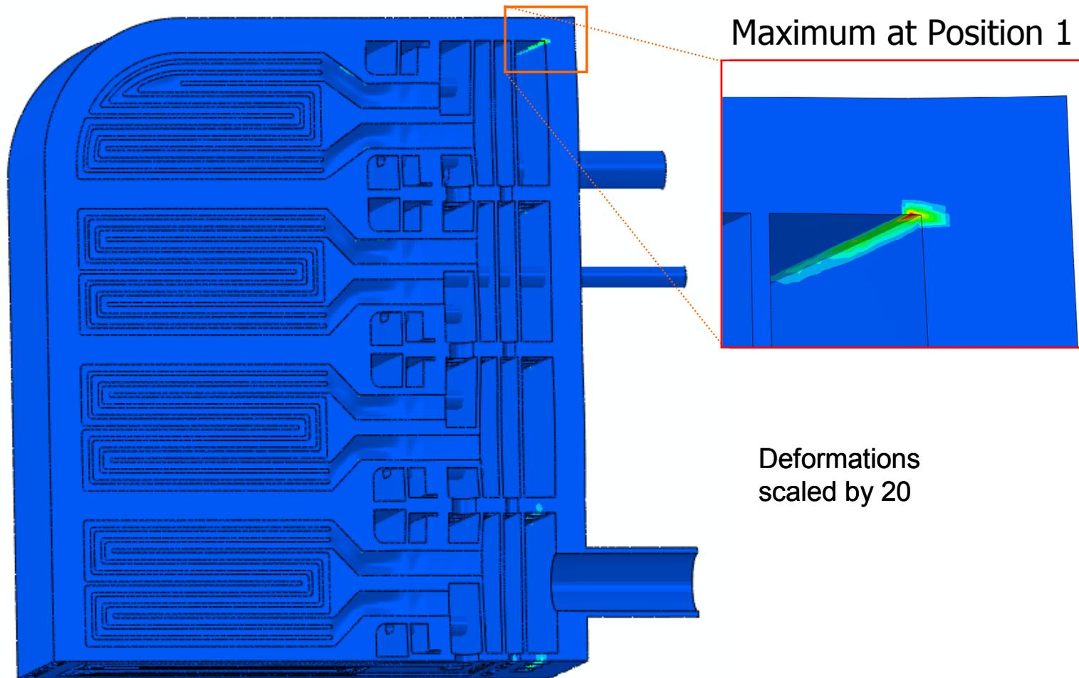
Distribution of "damage" due to fatigue and creep-fatigue in helium-cooled pebble bed test blanket module after 1st pulse with 400 sec dwell time.
