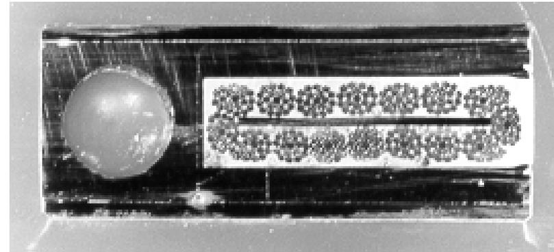
SULTAN 12T (2-stage flat cable, soldered to a brazed copper/steel stabilizer and pipe)
