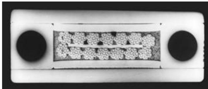
SULTAN 9T (2-stage flat cable, soldered to copper stabilizer, pipes and steel strips)
