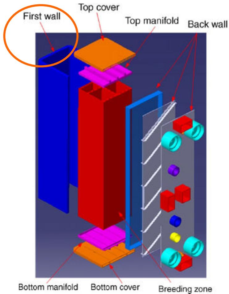
Fig. 3. The 3D model of HCML TBM.
