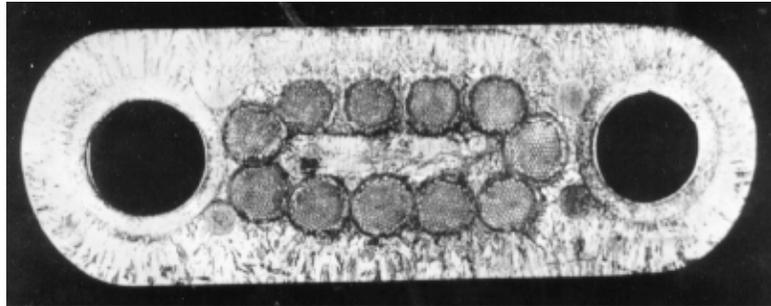
T15 (single stage, flat cable assembled by electro-plating to two copper pipes)
