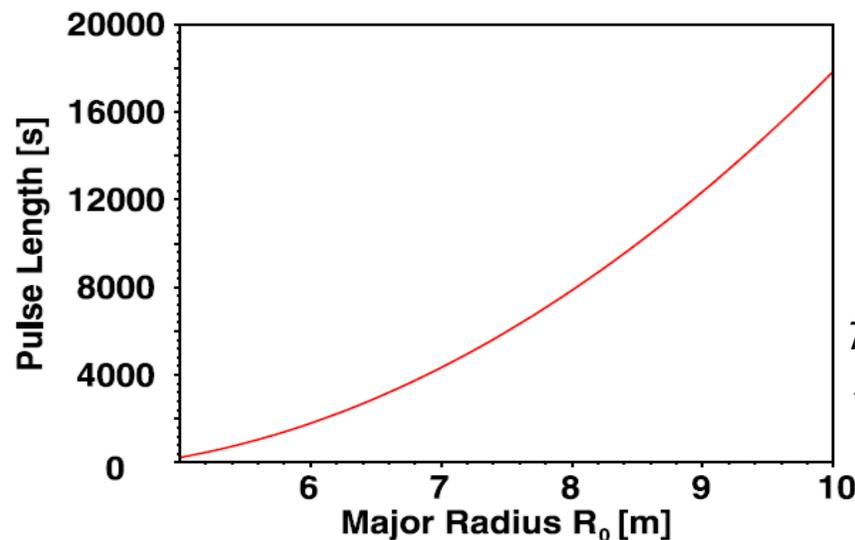
*T-pulse vs R for ITER-like machine with  $A=4$ ,  $B=7.4\text{T}$ ,  $\beta_N=2.6$  and  $f_{\text{CD}}=0$  (Zohm)*
