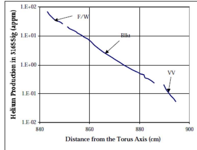
Figure 3.3-1b Helium production rate distribution in the outboard (in SS)
