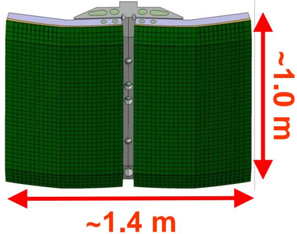
Plasma-facing surfaces: separable actively cooled with symmetric wings to shadow central access slot and protect against module-to-module misalignments (max. 5 mm)
