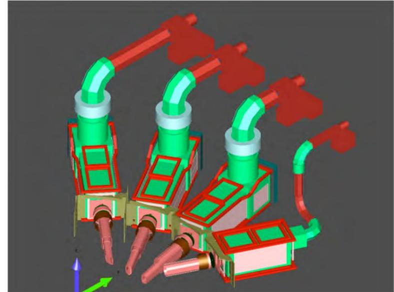
Fig. 36 3D view of MCNP geometry data (without concrete wall).
