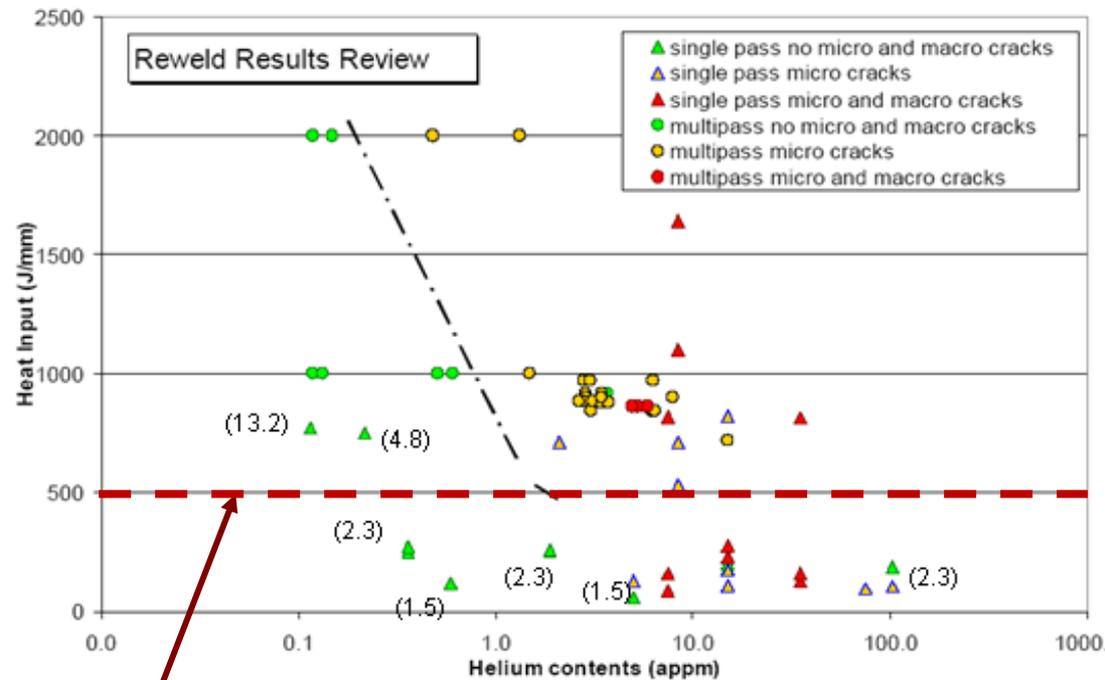
Limit for Laser and TIG for blanket pipe attachment
