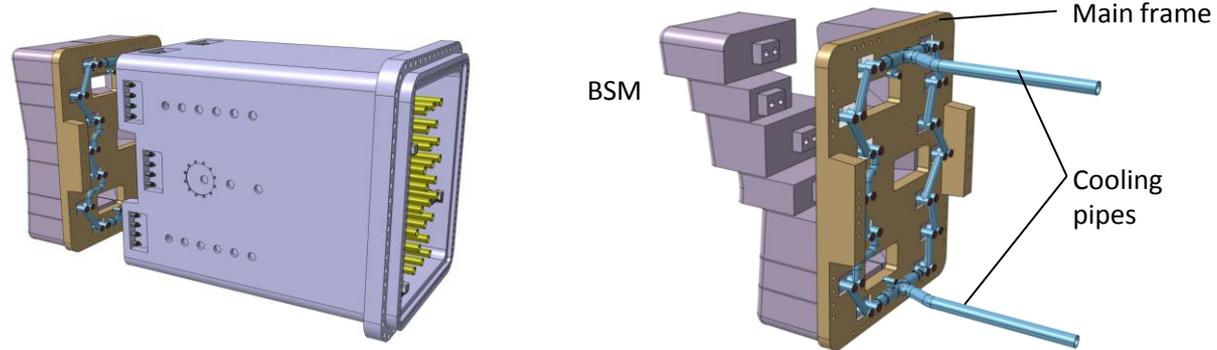
Modular approach for simplified replacement of assemblies and minimization of tasks.
