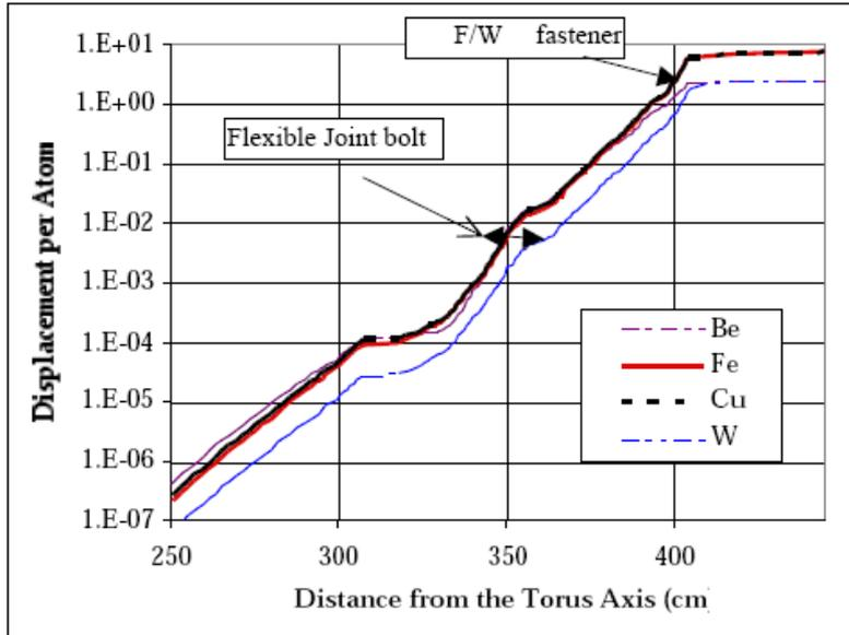
Damage in various material as a function of distance from the torus axis (inboard) [NAR]
