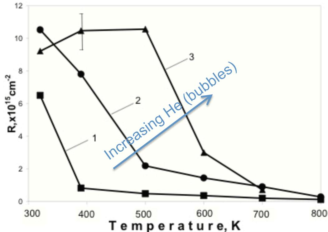
Fig. 8 Deuterium retention in 18Cr10NiTi steel implanted to  $1 \times 10^{16} \text{ cm}^{-2}$  without helium (1) and with helium to  $5 \times 10^{15}$  (2) and to  $5 \times 10^{16} \text{ cm}^{-2}$  (3).
