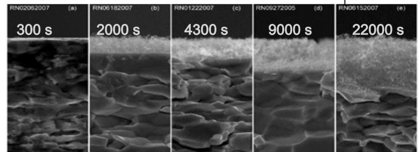
$$T_s = 1120 \text{ K}, \Gamma_{\text{He}^+} = 4\text{--}6 \times 10^{22} \text{ m}^{-2}\text{s}^{-1}, E_{\text{ion}} \sim 60 \text{ eV}$$
