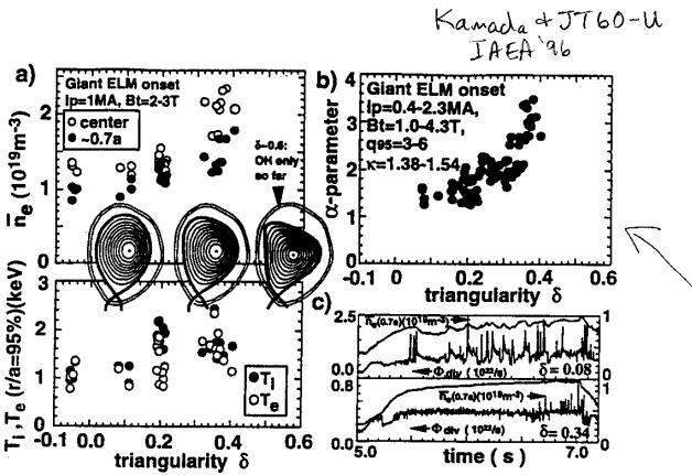
Fig. 1. a) and b): Increasing  $\overline{n}_e$  (center chord),  $\overline{n}_e$ (0.7a),  $T_e$ (r/a=95%),  $T_i$ (r/a=95%) and edge  $\alpha$ -parameter with increasing triangularity at onset of giant ELMs. c): Time traces of  $D_{\alpha}^{div}$  and  $\overline{n}_e$ (0.7a) for giant ELMs( $\delta$ =0.08) and grassy ELMs ( $\delta$ =0.34,  $\beta_p$ =2.4) with  $P_{NB}$ =20MW and  $I_p$ =0.6MA.
