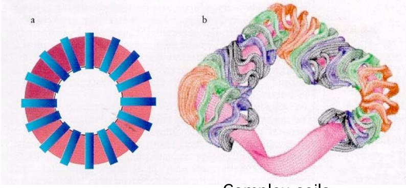
simple coils symmetric around axis current carrying Complex coils Helical symmetry within plasma
