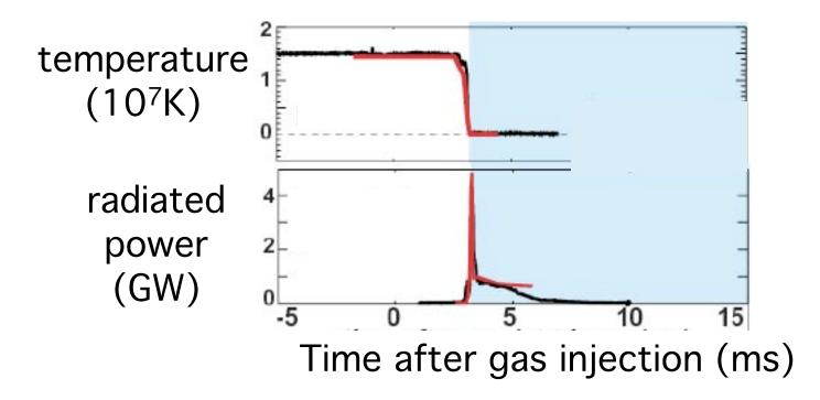
radiates nearly 100% of power in 200 microseconds, power radiated isotropically - no local damage
