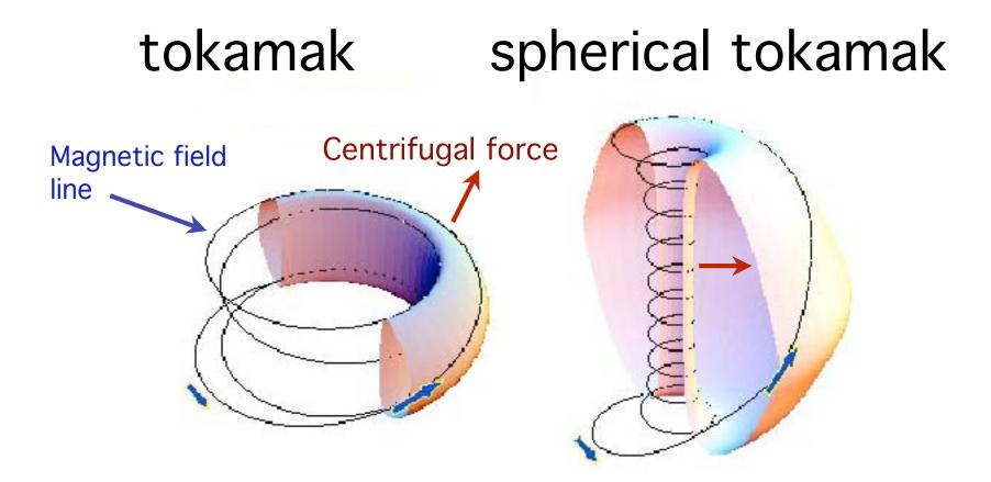
Instability from centrifugal force yields medium pressure Effect of centrifugal force weakened, yielding higher pressure
