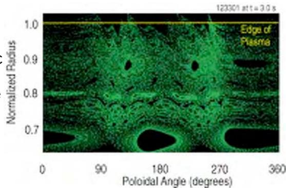
Unstable with high edge pressure gradients: sharp spikes in heat loss
