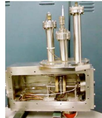
Pipe-Gun Pellet Injector
