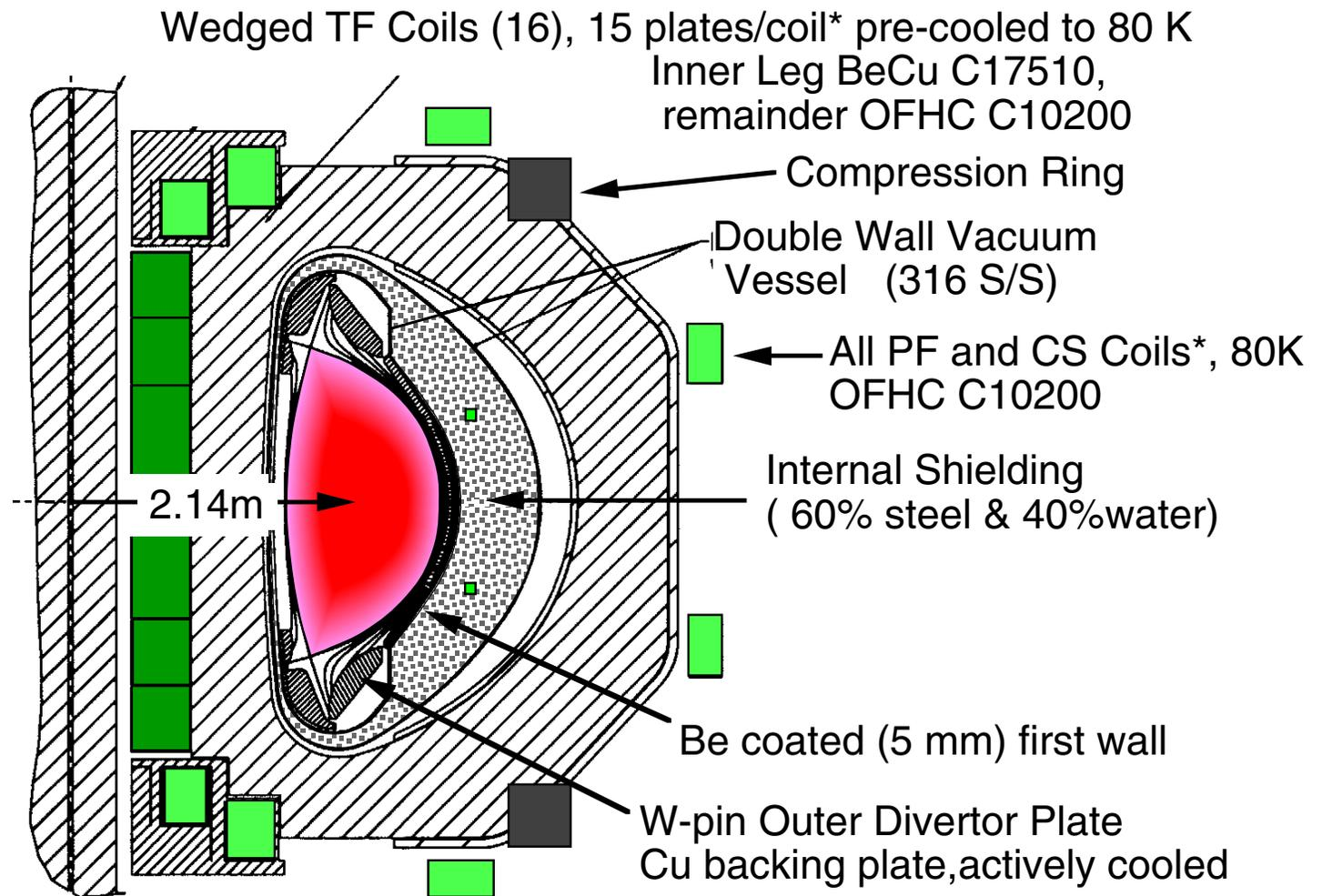
FIRE will push plasma facing components for the wall and divertor toward reactor power densities.
