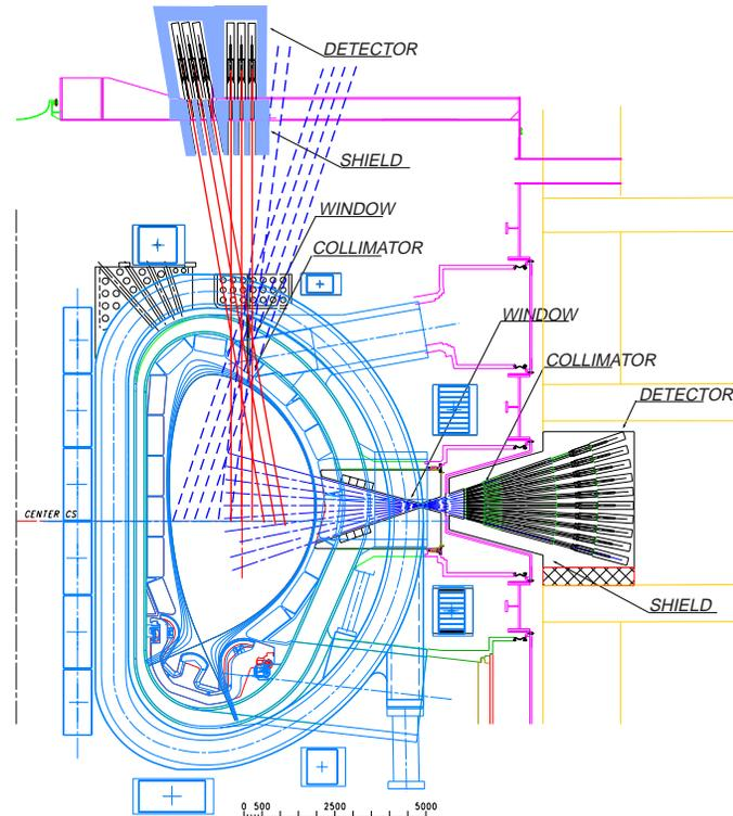
**Schematic of Radial and Vertical Neutron Cameras. The Sight-lines for the Vertical Camera will be distributed at Four Different Toroidal Locations [K Ebisawa et al, Rev. Sci. Instrum, vol. 72 No 1, 545, (2001)].**
