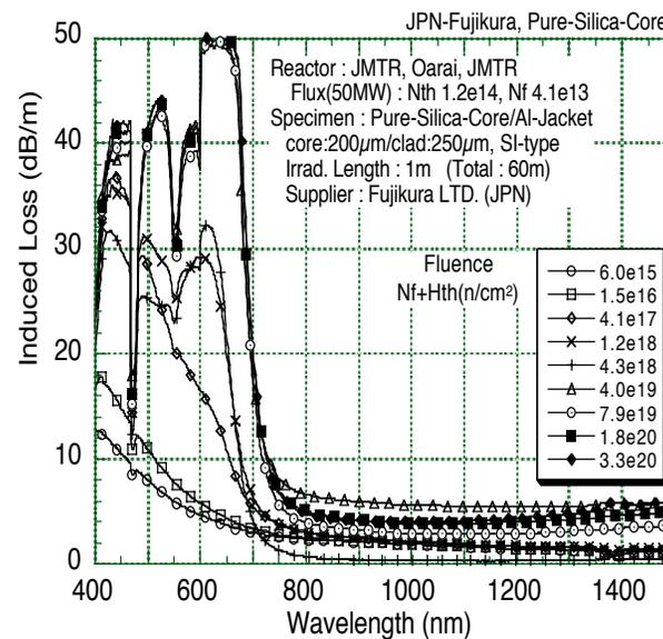
**Dose dependence of absorption of pure silica core fibre under fission neutron irradiation.**
