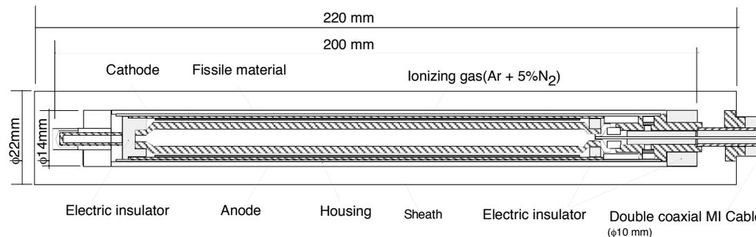
**Schematic diagram of typical microfission chamber. Fissile material, such as  $^{235}\text{U}$ , is coated on the cylindrical electrode. The ionizing gas between the electrodes is Ar + 5% N<sub>2</sub> (14.6 atm) [T Nishitani et al, Rev Sci Instrum 70 No 1 (1999) 1141]**
