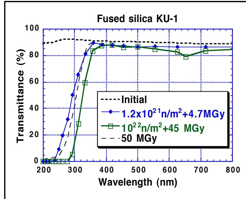
Measured transparency of KU1 fused silica (8 mm thick): as a function of wavelength for different neutron and gamma fluxes after irradiation in a nuclear reactor at  $T = 180^\circ\text{C}$  and with a  $\text{Co}^{60}$  gamma source at a room temperature [D.V.Orlinski. in J. Problems of Atomic Science and Engineering (in Russian), series – Nuclear fusion, v.2, 2000, p.21 – 39].
