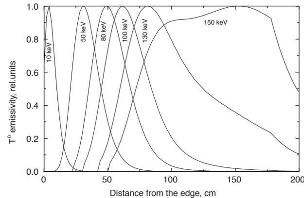
Calculated emissivity functions for T and typical ITER-FEAT conditions showing that with the upgraded NPA detector measurements of  $n_T/n_D$  should be possible into the central region [A.I.Kislyakov et al, in 'Diagnostics for Experimental Thermonuclear Fusion Reactors 2', ed. P.E. Stott, G. Gorini, and E. Sindoni, Plenum Press, New York, p.353 (1998)].
