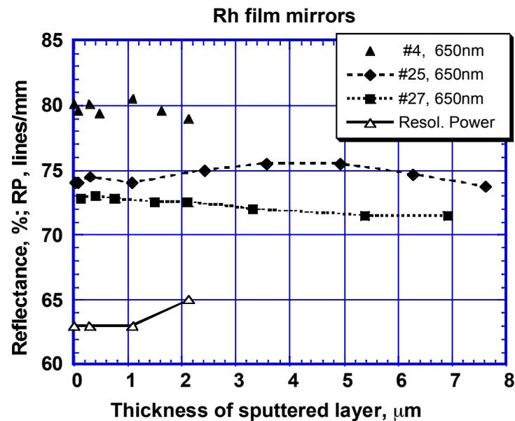
Dependences on sputtered layer thickness of reflectance at  $\lambda = 650 \text{ nm}$  and resolving power versus thickness of sputtered layer for Rh film on copper substrate mirrors. [V S Voitsenya et al, Rev. Sci. Instrum, vol. 72 No 1, 475, (2001)]
