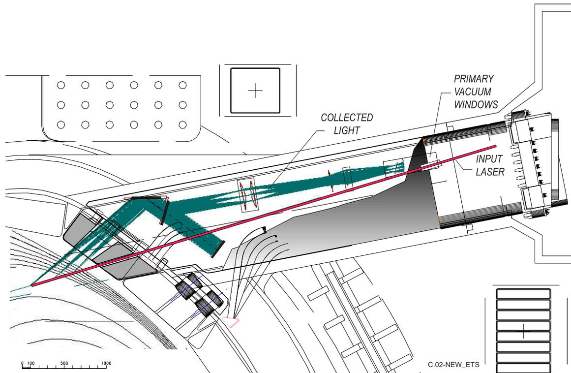
**Schematic of the Thomson Scattering System installed in an Upper Port**
