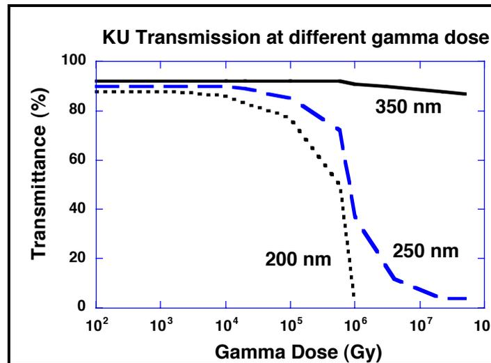
**Measured transparency of KU1 fused silica (8 mm thick): as a function of gamma dose at three wavelengths after irradiation with a Co<sup>60</sup> gamma source at a room temperature [D.V.Orlinski. in J. Problems of Atomic Science and Engineering (in Russian), series – Nuclear fusion, v.2, 2000, p.21 – 39].**
