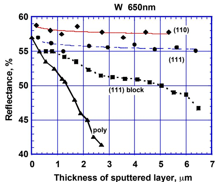
Reflectance of W mirrors (polycrystal, block monocrystal and real monocrystals with two planes of orientation) at  $\lambda = 650 \text{ nm}$  depending on the sputtered layer thickness. [V S Voitsenya et al, Rev. Sci. Instrum, vol. 72 No 1, 475, (2001)]
