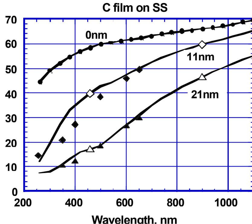
Experimentally measured (solid points) and calculated (lines with corresponding open markers) spectral dependencies of effective reflectance for clean SS and for SS with carbon coating of thickness indicated near every curve. [V S Voitsenya et al, Rev. Sci. Instrum, vol. 72 No 1, 475, (2001)].
