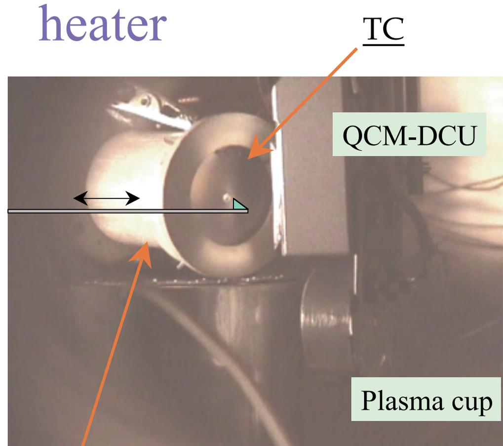
A HV heater was installed inside a BN cup.
