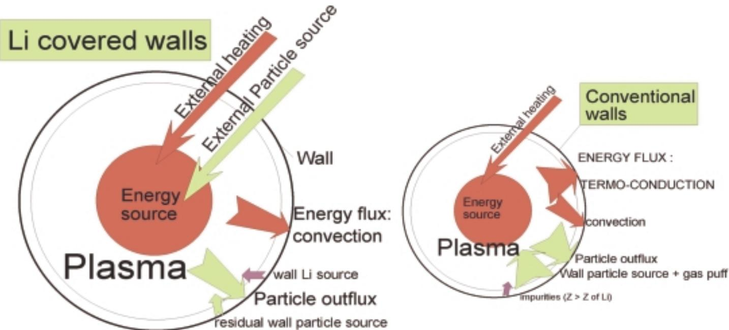
Lithium can be propelled along the walls for power and particle extraction.
