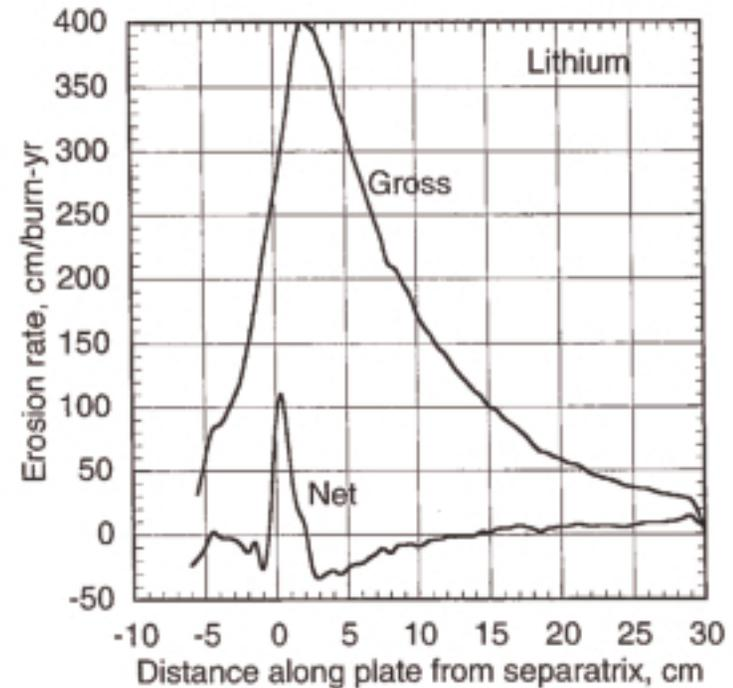
Gross and instantaneous (before liquid flow) net erosion rates from WBC code
