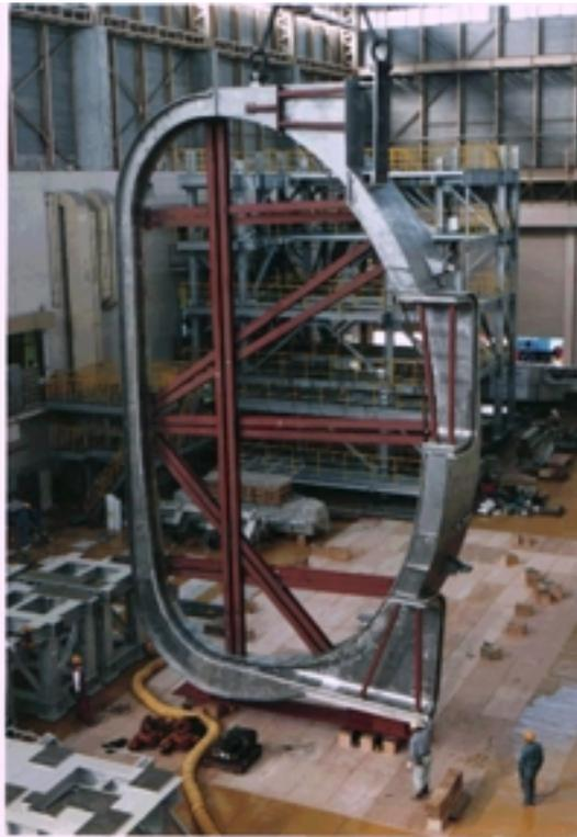
*Figure VI: Photograph of a the prototype sector of the vacuum vessel for ITER (Photo ITER).*
