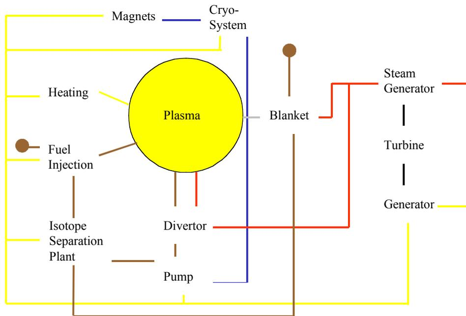
Figure III: Flow chart for a future fusion reactor: fuel (brown), electrical power (yellow), heat (red), neutron (grey), mechanical power (black) and cooled helium (blue).
