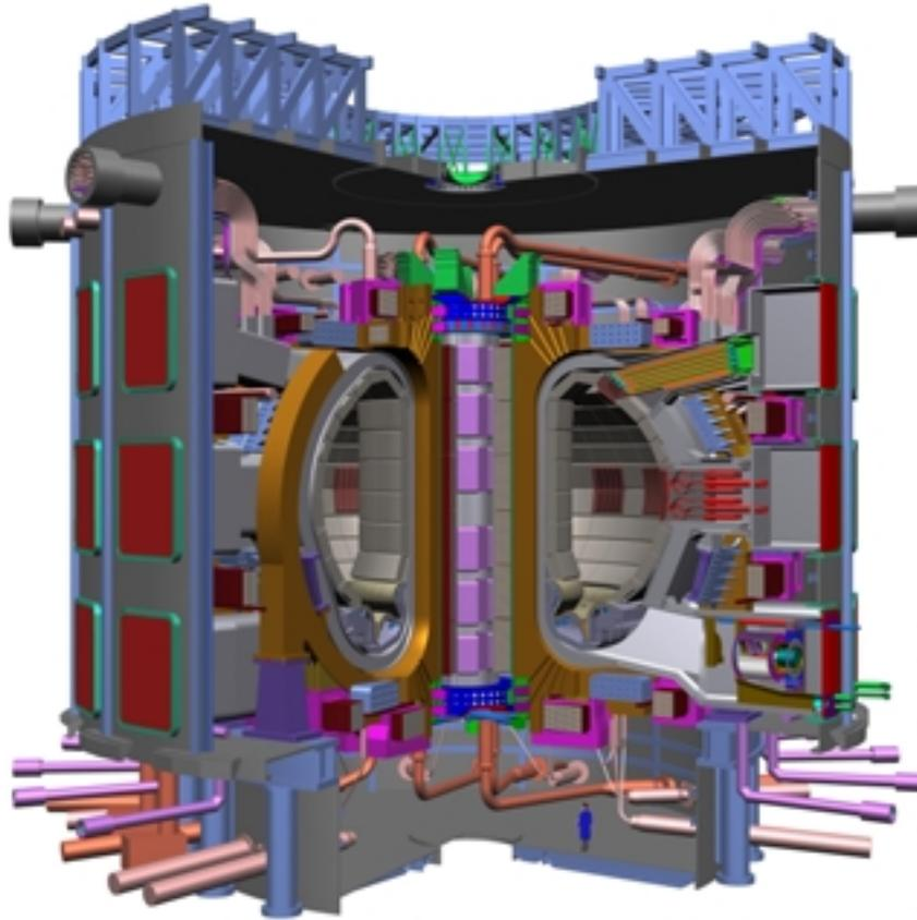
Figure VII: Sketch of the ITER-FEAT Experiment (photo ITER).
