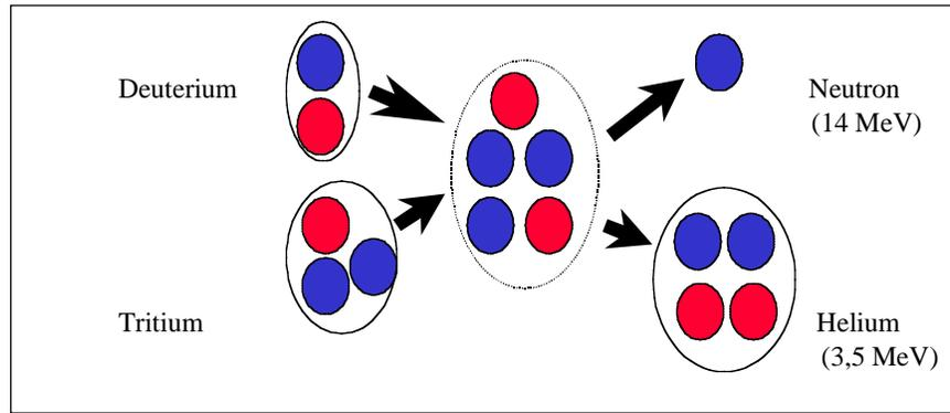
Figure 1: Schematic of the fusion reaction in which deuterium and tritium form a helium atom and a neutron. Mass is lost in the reaction and energy gained.
