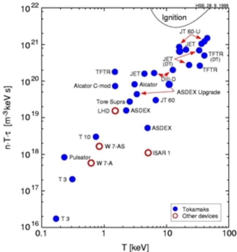
Figure IV: The development of the triple product of plasma temperature, plasma density and energy confinement time in the last three decades. The temperature 1 keV is equivalent to 11 Mio. K.
