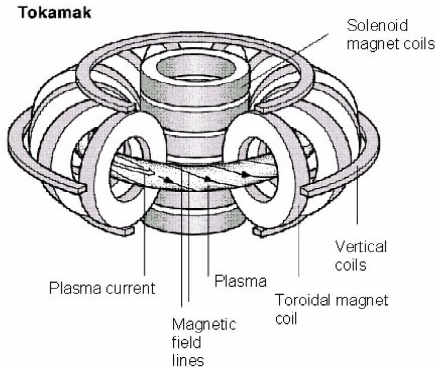
*Figure II: The tokamak has so far been the most successful magnetic confinement scheme. The magnetic field cage - necessary to confine the charged particles - is produced by the superposition of a toroidal magnetic field and a poloidal magnetic field produced by a current in the plasma.*
