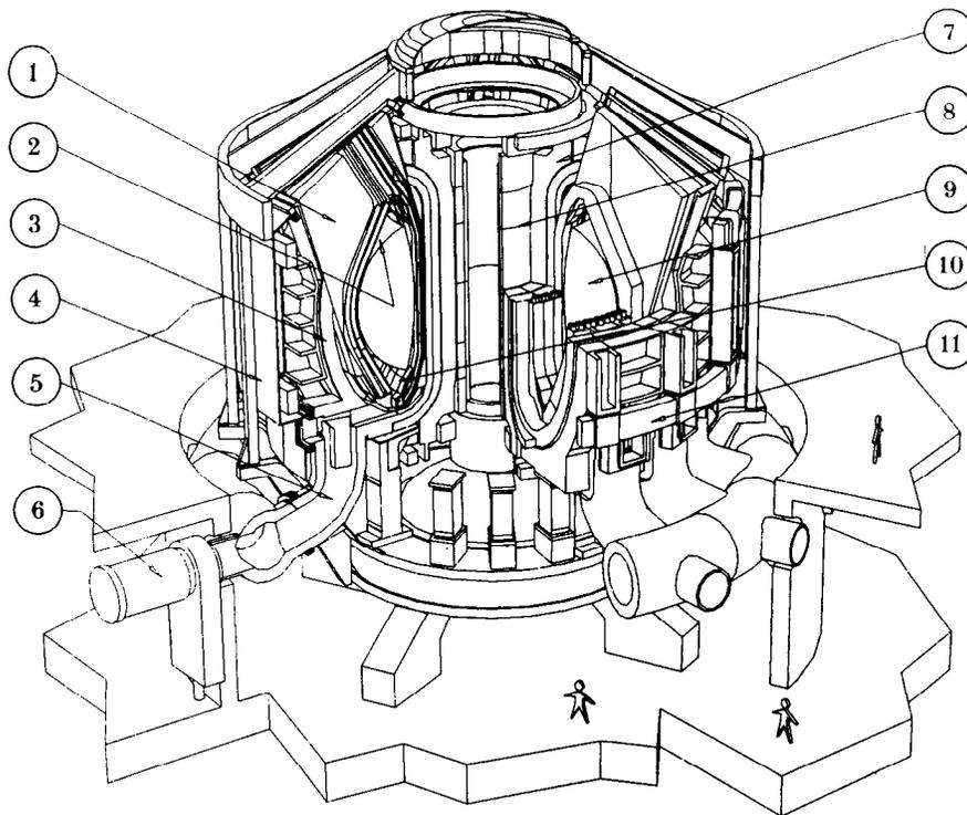
FIGURE 1. Sketch of NET-DN variant, showing (1) blanket, (2) first wall, (3) shield, (4) cryostat, (5) plasma exhaust duct, (6) vacuum pump, (7) toroidal-field coil, (8) inner poloidal-field coil, (9) plasma, (10) divertor plates, (11) outer poloidal-field coil.
