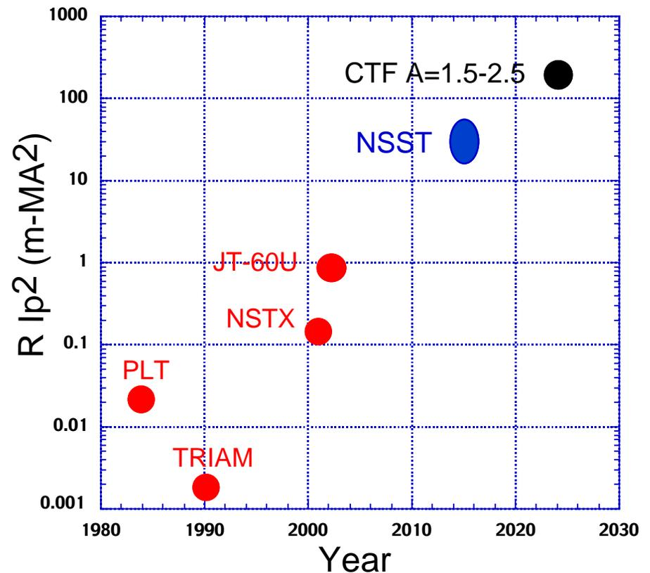
**NSST with 50 sec pulse length and  $R I_p^2 \leq 50$  m-MA<sup>2</sup> is designed to be a good test bed for such demonstration.**
