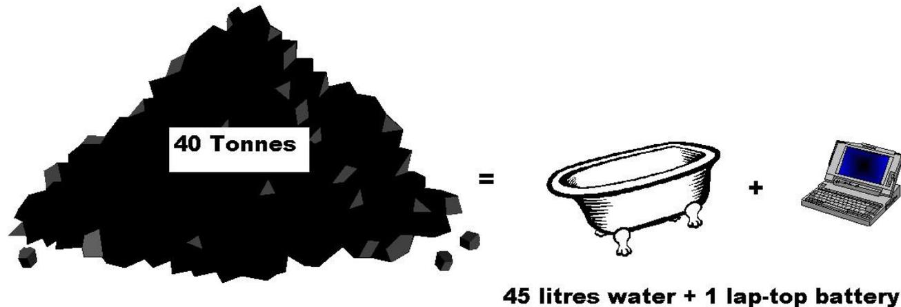
Lithium in one laptop battery + half a bath-full of ordinary water ( $\Rightarrow$  one egg cup full of heavy water)  $\longrightarrow$  200,000 kW-hours
