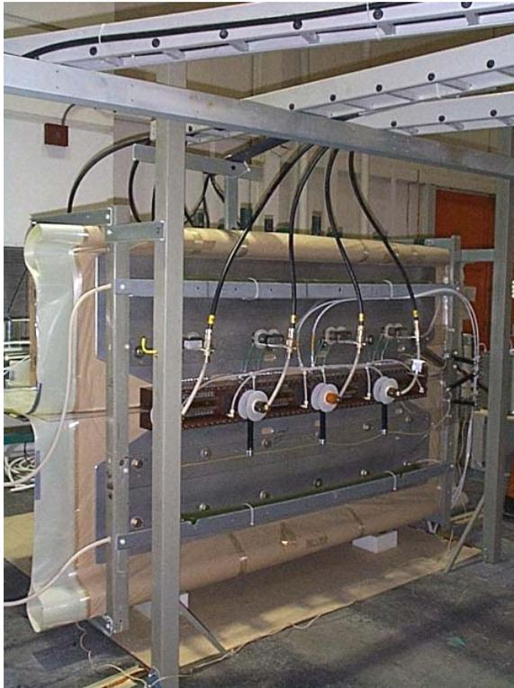
Back view of the Main bank showing the Crowbar switch and the RG 17/14 transmission line cables to run to the Theta-coil-cable header.
