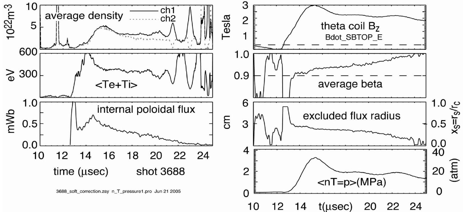
FRC parameters in FRX-L, following installation of improved high-current crowbar system. The plasma pressure is 2-3 MegaPascals, (20-30 bars); higher than even the highest field tokamak plasmas. An  $n=2$  rotational instability develops by  $t=20 \mu\text{sec}$ , terminating the plasma.
