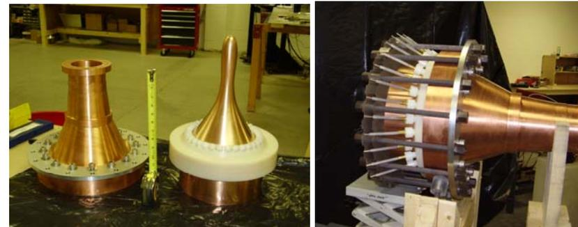
Full-scale accelerator module with 32 capillary injectors built and tested. Unit shown will be installed on MCX at University of Maryland
