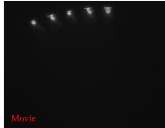
5 capillary injectors firing simultaneously into 60 mTorr vacuum at 10.8 km/s. Obtained from PI-Max camera using 50 ns gate shutter with 500 ns between frames.
