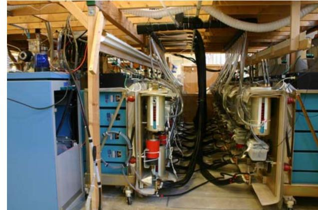
Fast energy storage 300 kJ at +/- 25 kV in 12 pairs of individually charged and triggered modules.
