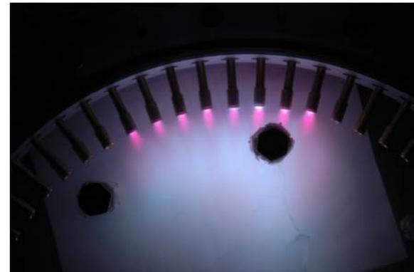
Multiple jets firing in visible light. 1 second exposure. Dark blotches in field of view are external bolts.
