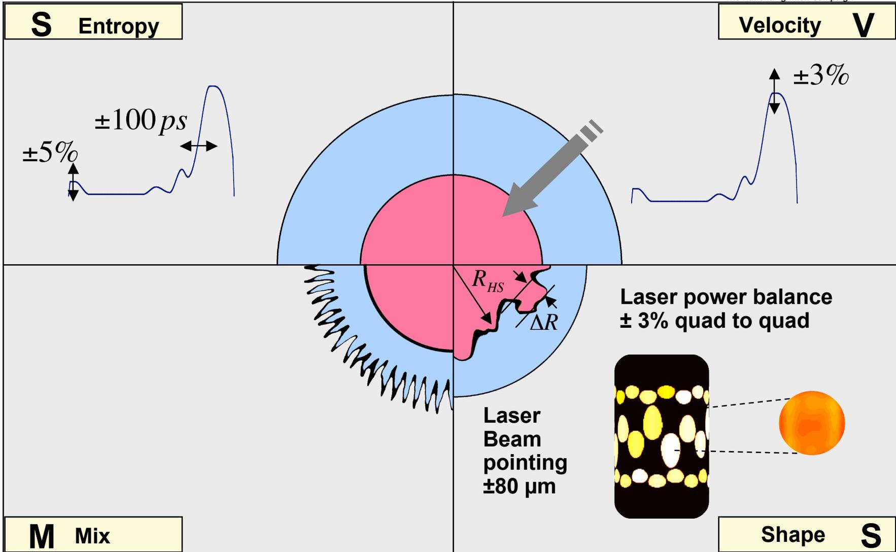
To compensate for physics uncertainties the laser and target parameters must be experimentally tuned
