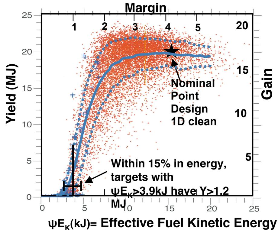
$$\text{Margin} = \frac{E_{fuel}}{3.9kJ} * \psi = \frac{E_{fuel}}{3.9kJ} \left( \frac{\langle v \rangle}{365km/sec} \right)^{5.9} \left( \frac{\langle \alpha \rangle}{1.46} \right)^{-3.9} \left( 1 - \frac{\Delta R_{hotspot}}{R_{hotspot}} \right)^{3.5} \left( 1 - \left[ \frac{0.5\Delta R_{mix}}{\Delta R_{shell}} \right] \right)$$
