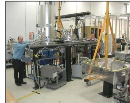
Fill targets & layer in a cryogenic fluidized bed
