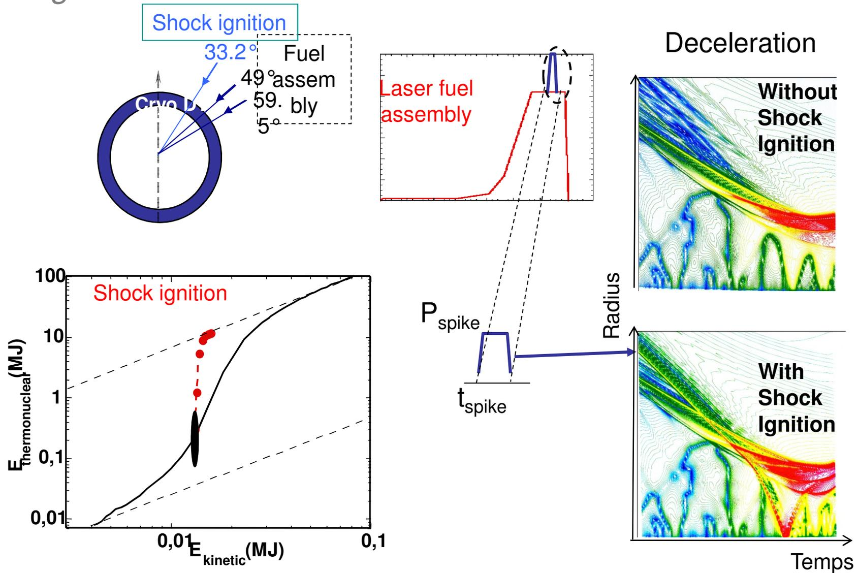
$(\alpha=2, v=400\text{km/s})$ -Direct-drive marginally igniting target can be shock ignited with high gain.
