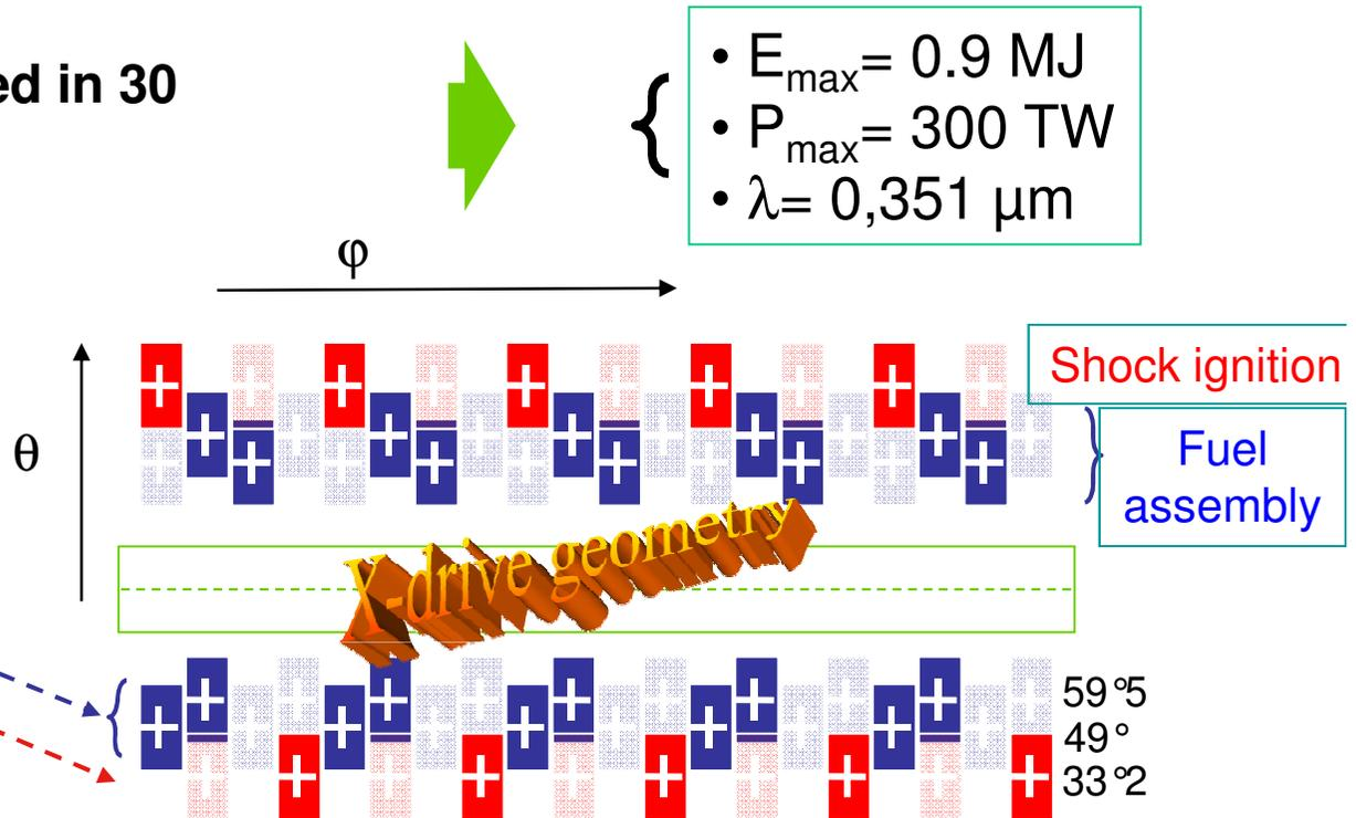
Direct-drive fuel assembly is still done with beams at  $49^{\circ}$  and  $59^{\circ}5$  WITHOUT PDD (\*).
