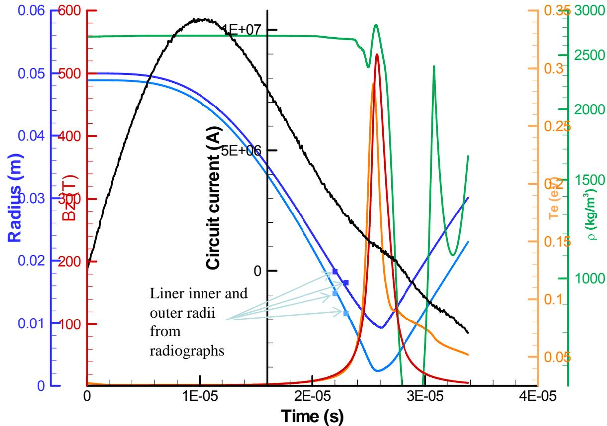
NumerX MACH2 results for Shiva Star liner compression for 2 Tesla initial axial magnetic field
