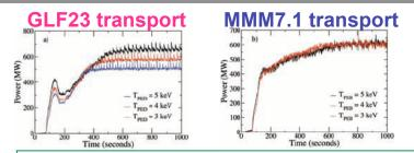
TSC/PTRANSP simulation of ITER 15MA fusion performance for two transport models (T. Rafiq et al., 2011)
