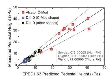
Comparison of EPED (v1.63) model for the H-mode pressure pedestal height with data from Alcator C-Mod and DIII-D. (J. Hughes et al. 2011)
