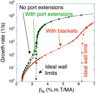
VALEN modeling of RWM growth rate in ITER showing effects of structural elements (J. Bialek, 2011)
