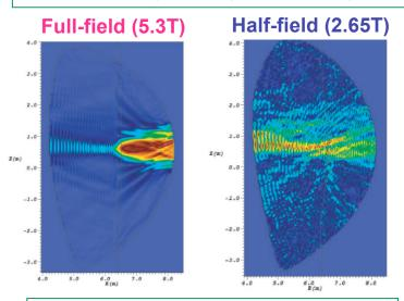
AORSA code modeling of RF wavefields for ITER reference scenarios (R. Budny et al., 2011)
