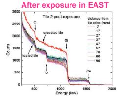
Rutherford backscattering analysis of a tile with a 1µm C layer following erosion by >10hr plasma exposure in EAST tokamak (W. Wampler, 2011)
