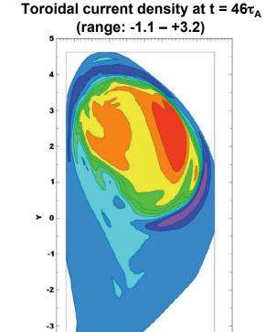
M3D modeling of an ITER VDE-triggered disruption (H. Strauss, 2011)
