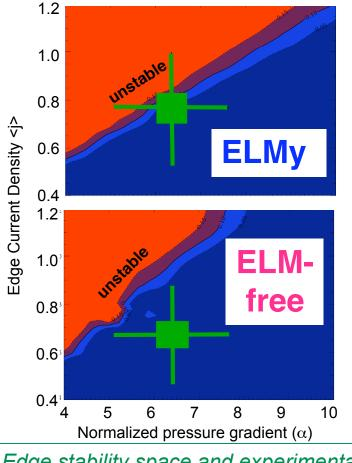
Edge stability space and experimental data for ELMy (non-lithium) and ELM-free (with-lithium) NSTX discharges (D. Boyle, 2011)
