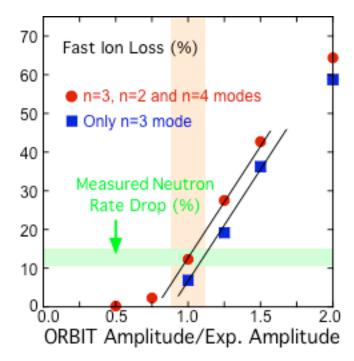
Fast ion transport modeled in ORBIT using linear NOVA eigenmodes, empirical amplitude and frequency evolution. The sharp threshold for loss onset is consistent with the avalanche model. (E. Fredrickson et al. 2011)
