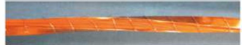
Tapes are stacked with copper strips, and then twisted.
