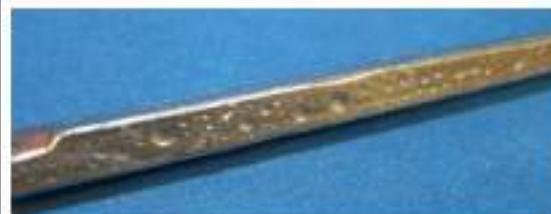
Square (5.8 mm x 5.8 mm) soldered conductor
