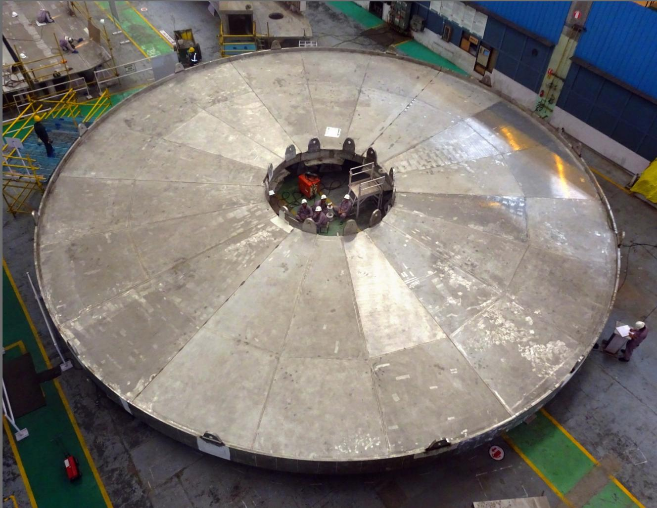
India is responsible for the fabrication and assembly of the 30 x 30 meter ITER cryostat. Pictured, six 60° base plates are temporarily assembled at the factory in order to check tolerances prior to shipment to the ITER site.
