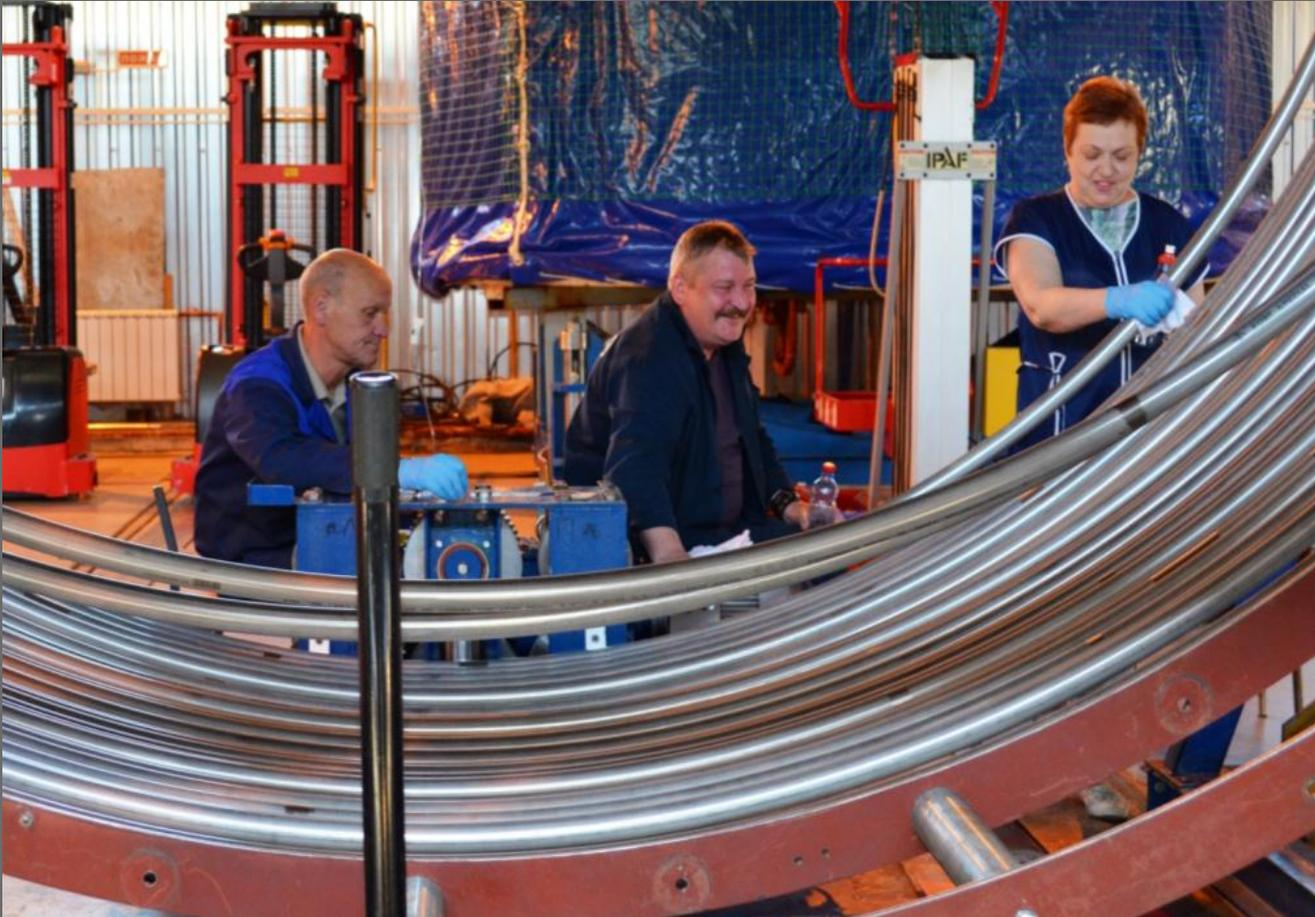
Russia completes its share of toroidal field conductor in June 2015. The milestone marks the end of a five-year campaign to manufacture 28 production lengths (more than 120 tons of material).
