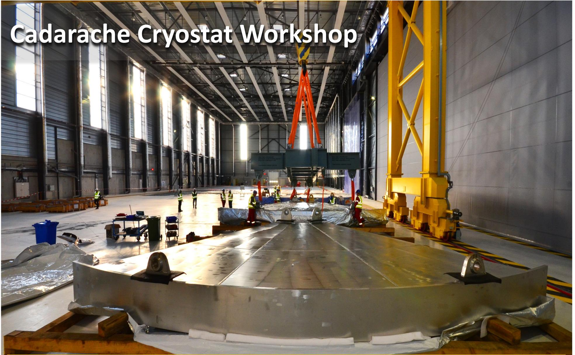
The Indian Domestic Agency has erected the Cryostat Workshop for assembly of the 30 x 30 metre cryostat, that will completely enclose the ITER Tokamak. The first cryostat elements, shown here, arrived at ITER last week. The remainder of the cryostat base will arrive tomorrow, 17 December, achieving the first Milestone ahead of schedule.
