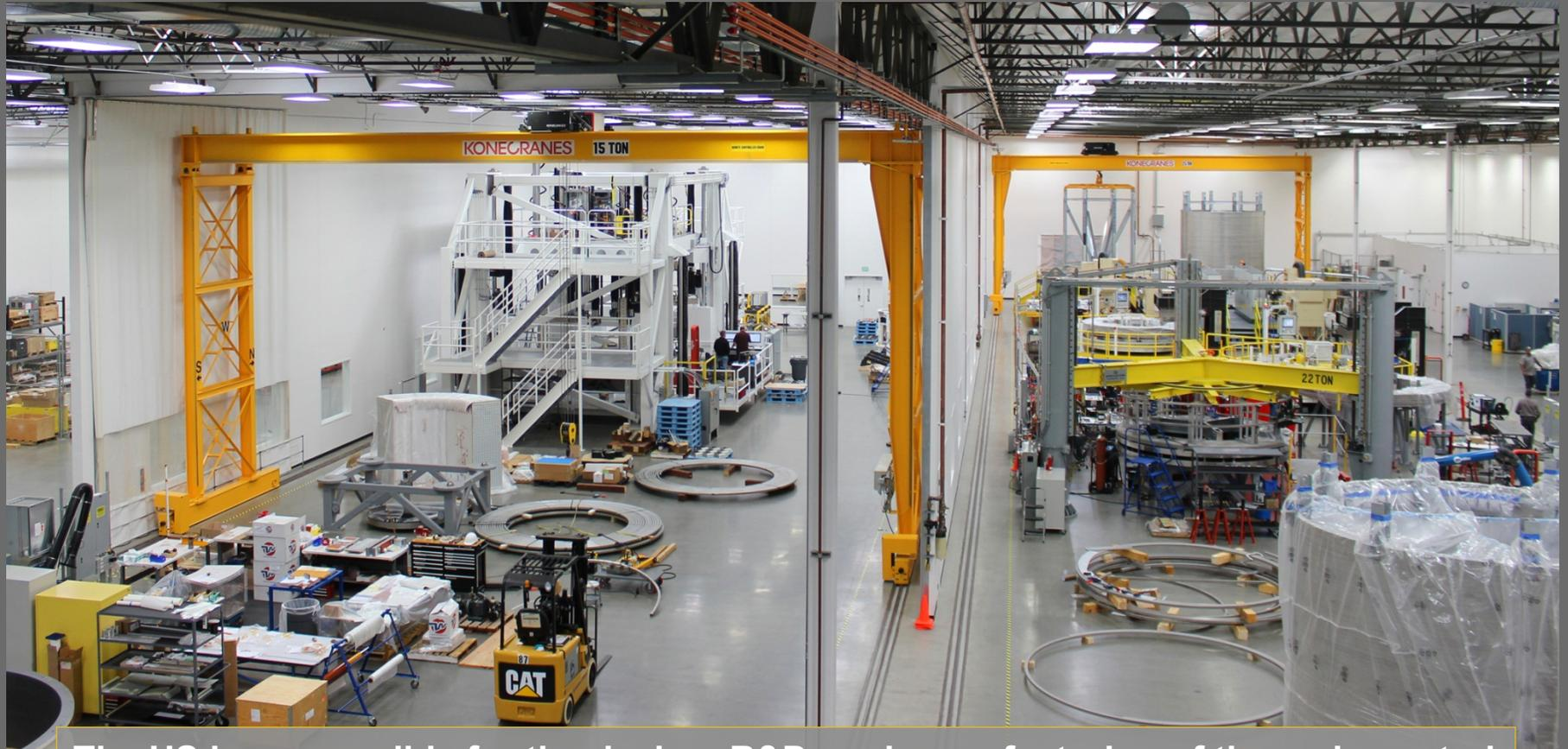
The US is responsible for the design, R&D, and manufacturing of the main central solenoid magnet (using conductor supplied by Japan), as well as the associated structure and tooling. At General Atomics' Magnet Technologies Center in Poway, California, winding operations began in April 2015 on a mockup module.
