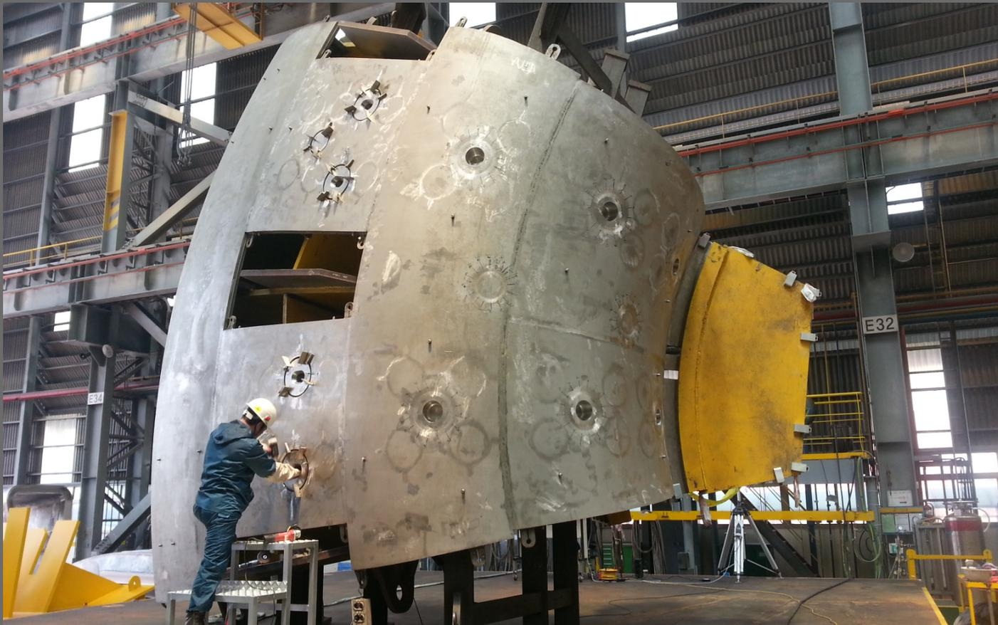
In Korea, where two of nine vacuum vessel sectors are under construction, welding is carried out on the upper section of an inner shell—only a small piece of the full component.
