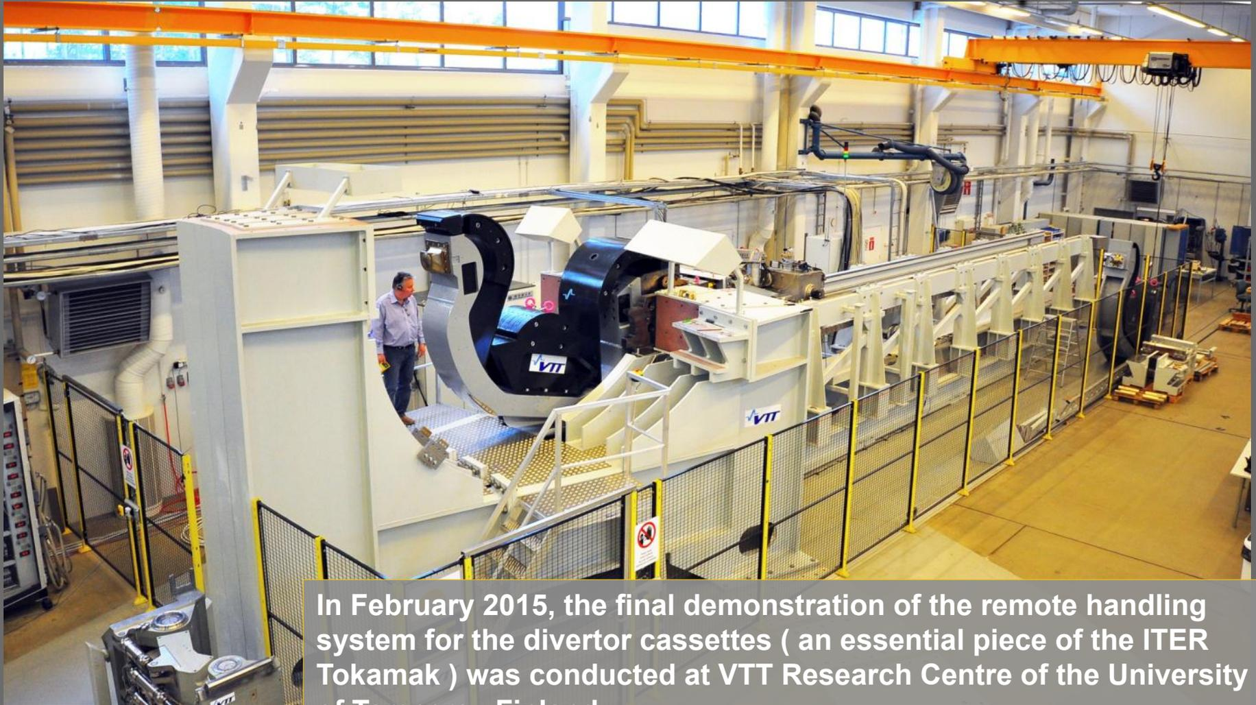
In February 2015, the final demonstration of the remote handling system for the divertor cassettes ( an essential piece of the ITER Tokamak ) was conducted at VTT Research Centre of the University of Tampere , Finland.
