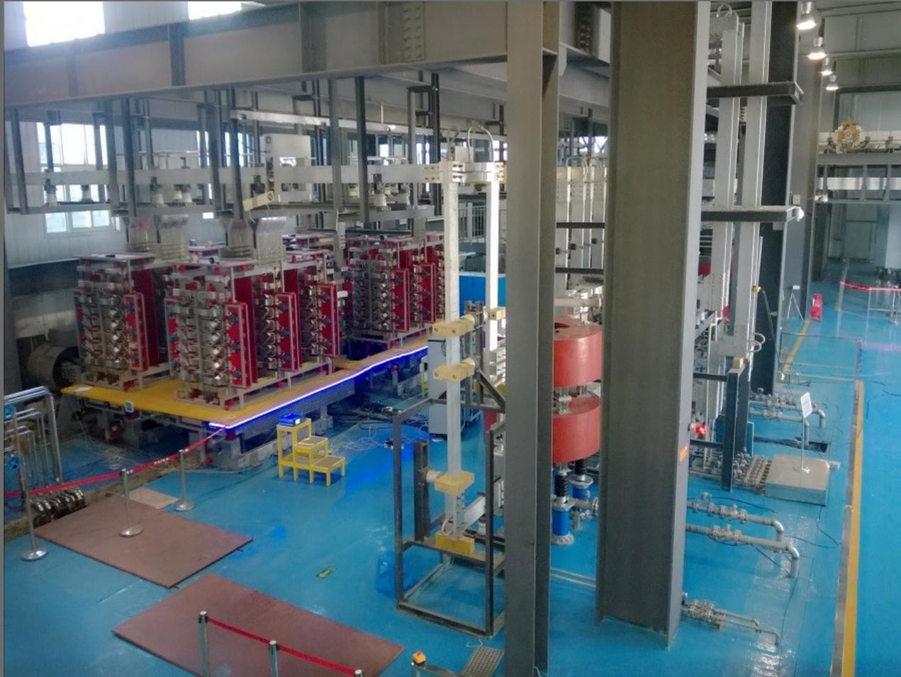
China is responsible for the procurement of 14 poloidal field AC/DC converter units that will provide reliable, controlled DC power to the ITER poloidal field magnetic coils. The testing of a prototype converter unit opens the way to future batch production.
