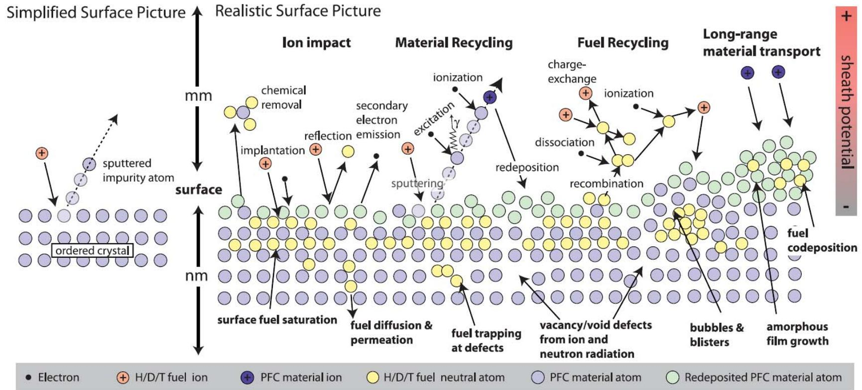
Comparison of a simplified plasma/surface model where only sputtering occurs (left) with a realistic model (right) where many types of interactions occur within the material during bombardment by a fusion plasma. From B. Wirth.
