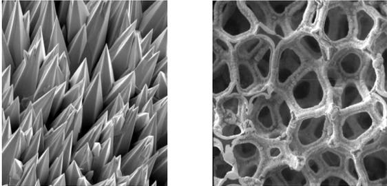
Ultramet adapted previous work on foam-core heat exchangers for plasma-facing components, to construct a high temperature heat exchanger to enhance heat transfer between liquid lithium and helium. The heat exchanger would be used for fission-based power systems for lunar and planetary surface bases.
