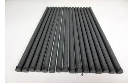
Fusion materials science researchers developed highly radiation-tolerant silicon carbide ceramic composites for nuclear thermo-structural applications. These composites are now central to the accident-tolerant fuels and core technologies, which are being developed for the current and next generation nuclear reactors to survive the severe accidents.
