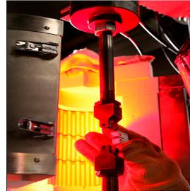
ORNL researchers developed a new cast stainless steel that is 70 percent stronger than comparable steels. These alloys will help engine manufacturers meet emission regulations for diesel, turbine, and gasoline engine applications.
