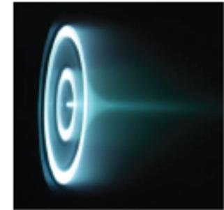
Plasma thrusters make use of LTPs for space propulsion. Thrust is achieved through the expulsion of ions at high energy. Unlike chemical rockets, plasma thrusters use an electrical power source. Plasma thrusters are in current use for maneuvering of near earth satellites, and are under development for interplanetary missions.
