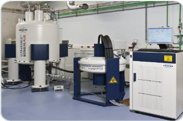
Using high frequency microwaves enables the polarization of the electron spin system, eventually leading to polarization of the nuclear spins in a process known as Dynamic Nuclear Polarization (DNP NMR). The increase in signal to noise ratio can be several hundred, an enormous enhancement allowing experiments to be completed in days rather than months.
