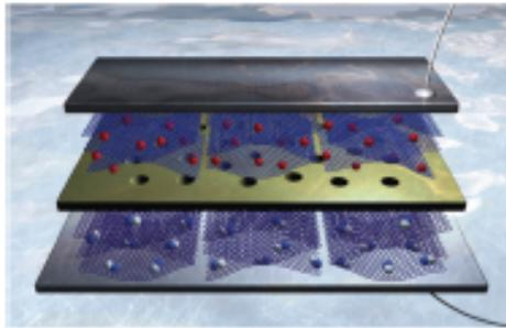
Plasma deposition and etching processes are used to create graphene structures with remarkable electrical and thermal properties. For many applications, batteries for energy storage may be replaced. Supercapacitors with a single graphene layer charge quickly and have a long life.
