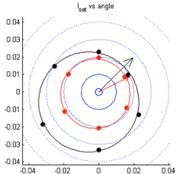
$$I_{\text{sat}}(\theta) = A \exp\left(\left(\frac{M}{2}\right) \left[.64(1 - \cos(\theta - \theta_F)) + .7(1 + \cos(\theta - \theta_F))\right]\right)$$
