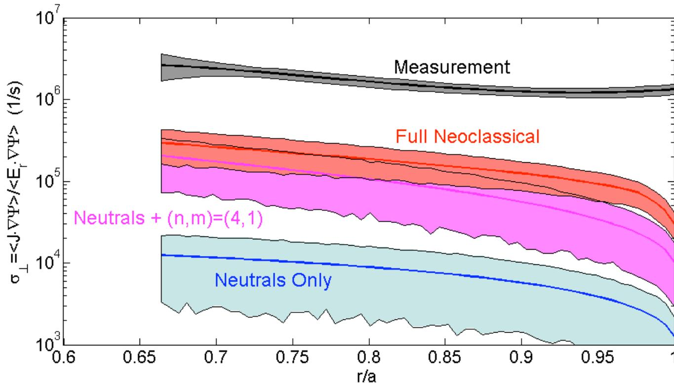
$$\langle \bar{J}_{\text{plasma}} \cdot \bar{\nabla} \psi \rangle = \sigma_{\perp} \left( \langle \bar{E}_r \cdot \bar{\nabla} \psi \rangle - \frac{\langle \bar{\nabla} p_i \cdot \bar{\nabla} \psi \rangle}{eN_i} \right)$$
