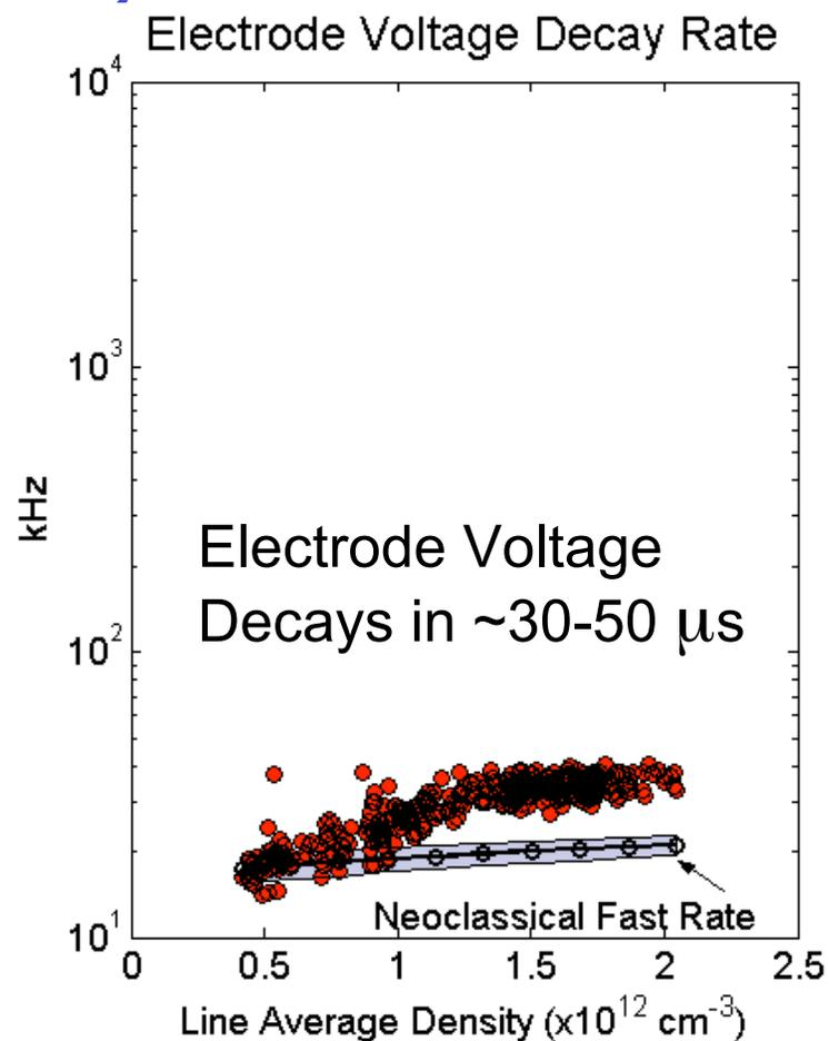
**Floating potential and fast component of flow decay on same time-scale as electrode voltage, in agreement with neoclassical fast rate.**
