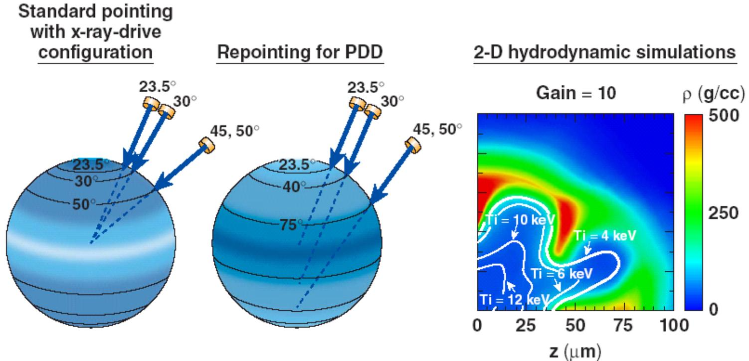
Polar direct drive is based on the optimization of phase-plate design, beam pointing, and pulse shaping (S.P.Regan, OV-3/3).
