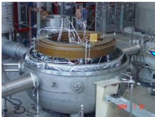
One set divertor coil inside the cryostat of the test facility
