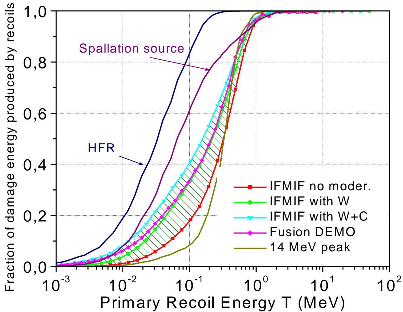
Fig. 2: The IFMIF high flux region meets perfectly (hatched area) DEMO relevant conditions
