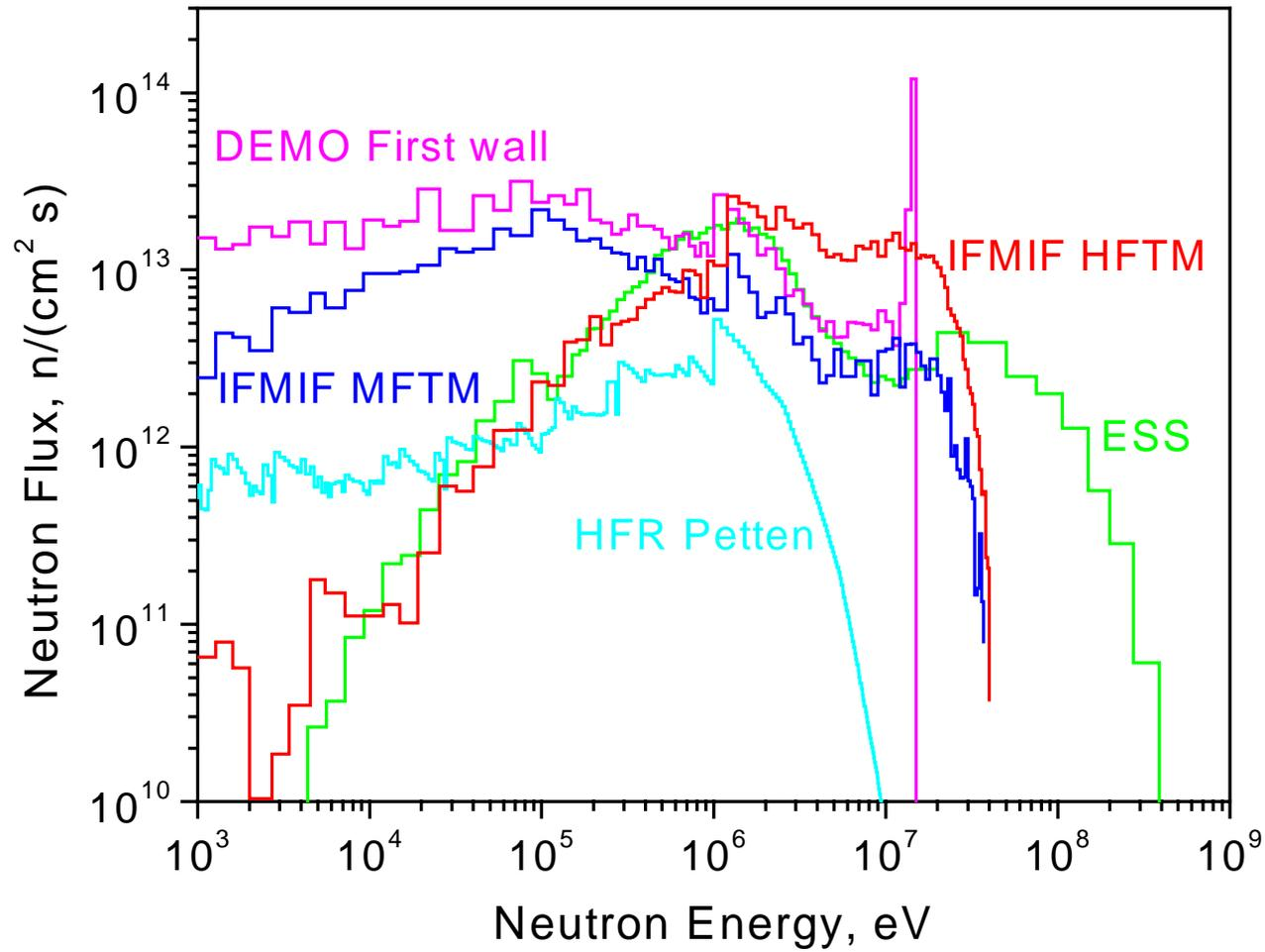
Fig. 1: Typical neutron spectra of (i) DEMO First Wall (HCPB Blanket), (ii) mixed spectrum reactor HFR Petten, (iii) European Spallation Source, (iv) IFMIF High flux test module, and (v) IFMIF medium flux test module.
