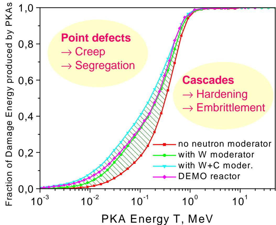
DEMO-relevant PKA spectra can be perfectly adjusted with neutron moderators & reflectors
