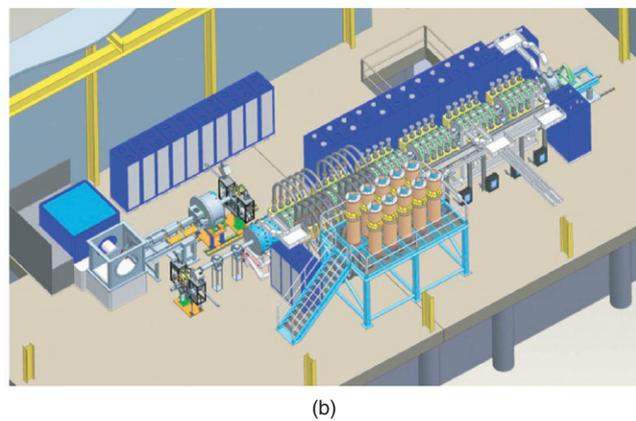
**Figure 7.** (a) Design of the fast ignition power plant. It is driven by a diode-pumped solid-state laser operated with 16 Hz/1.1 MJ. The system consists of four reactor chambers. Each chamber is operated with 3 Hz. The total output electric power is about 1200 MW (Norimatsu T. *et al* 2007). (b) A heavy ion beam driver is developed at LBNL as the HIBF virtual laboratory of USA. This will be the test bed of the high power heavy ion beam accelerator.
