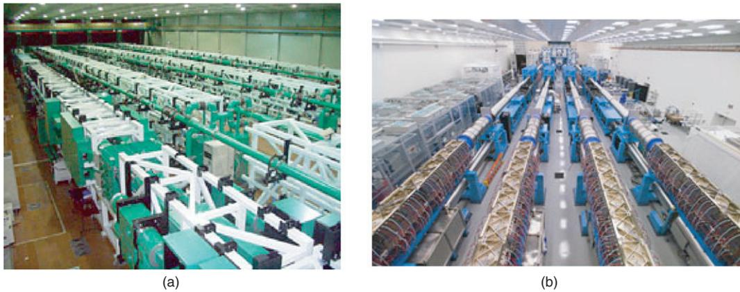
**Figure 6.** Two integrated fast ignition experimental machines. (a) The LFEX laser (10 kJ/a few picoseconds heating laser) together with the GXII laser. (b) The OMEGA-EP laser (two beam system, 5 kJ/a few picoseconds).
