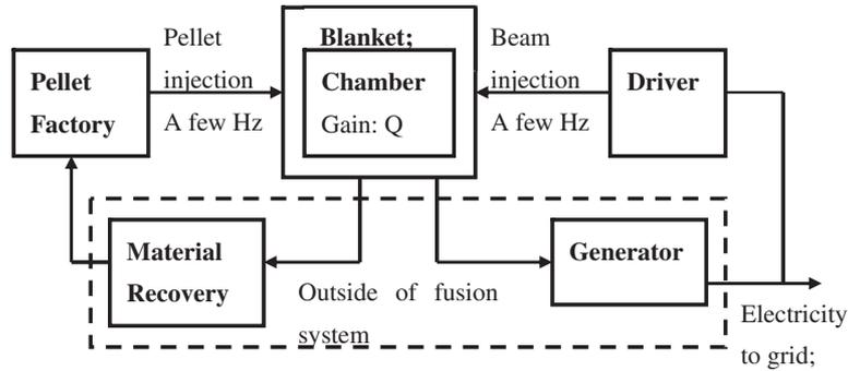
Figure 1. Energy and material flow diagram in laser fusion power reactor.
