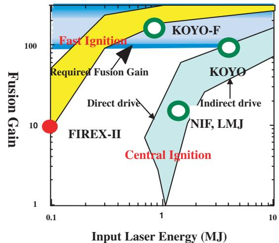
**Figure 4.** Predicted fusion gain for central ignition and fast ignition. NIF and LMJ are the ignition demonstration facilities for the central ignition. FIREX-II is the planned facility for the demonstration of fast ignition.
