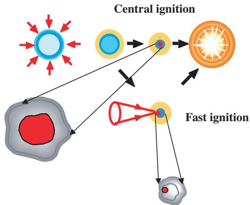
**Figure 5.** Central ignition and fast ignition. The plasma density of the hot spark in fast ignition is expected to be 3–5 times higher than that for central ignition. Therefore, the hot spark size indicated by the red area is much smaller in fast ignition. Thus, the required laser energy for ignition and high gain will be smaller by one order of magnitude.
