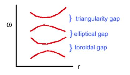
m and m+3 are now coupled and an triangularity "gap" is opened in the continuous spectrum
