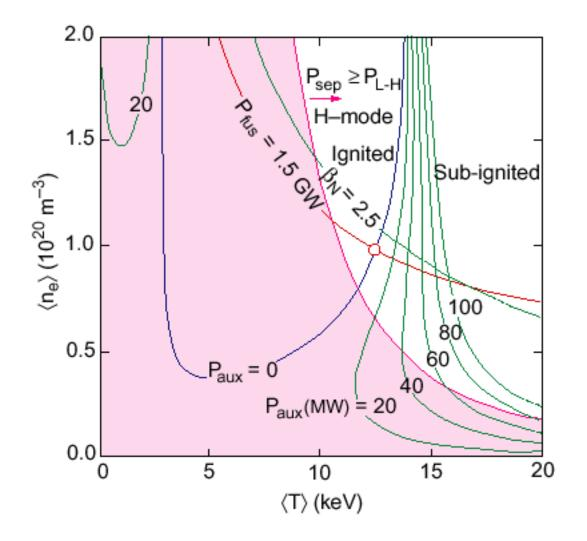
Additional limits on density, pressure, & power thresholds constrain operating space.
