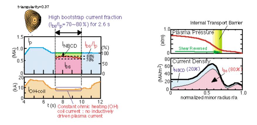
Data from JT-60U shows sustained transport barrier and 100% non-inductive current drive PLASMA BOUNDARY PHYSICS: HEAT REMOVAL & CONFINEMENT
