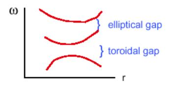
m and m+2 are now coupled and an elliptical "gap" is opened in the continuous spectrum
