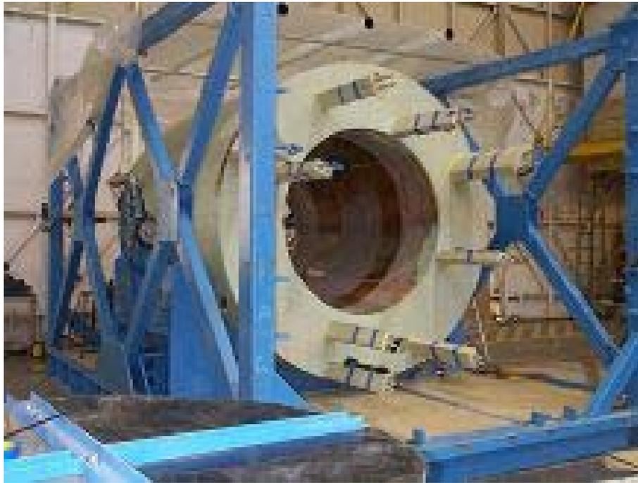
Figure 3.7 ITER Central Solenoid Model Coil that achieved 13 T and x.x T/s ramp rate (1/2 scale of full coil). Courtesy of ITER.
