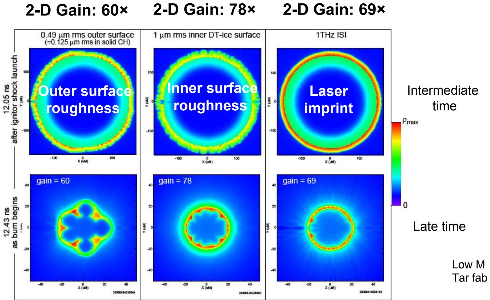
250 kJ shock ignited target – NRL FASTERAD3D simulations
