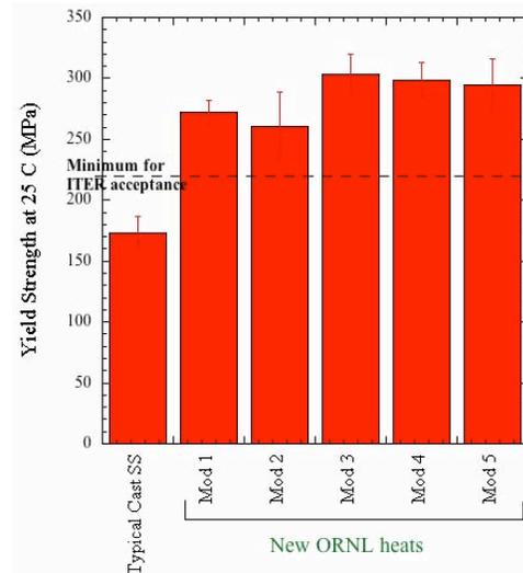
Tensile tests at 25°C
