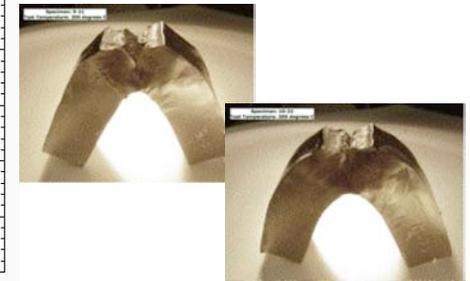
Impact testing at 200-300°C. Samples do not break.
