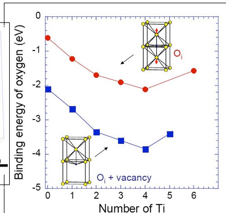
The presence of Ti and vacancy has a drastic effect in lowering the binding energy of oxygen in Fe (C. L. Fu and M. Krcmar).
