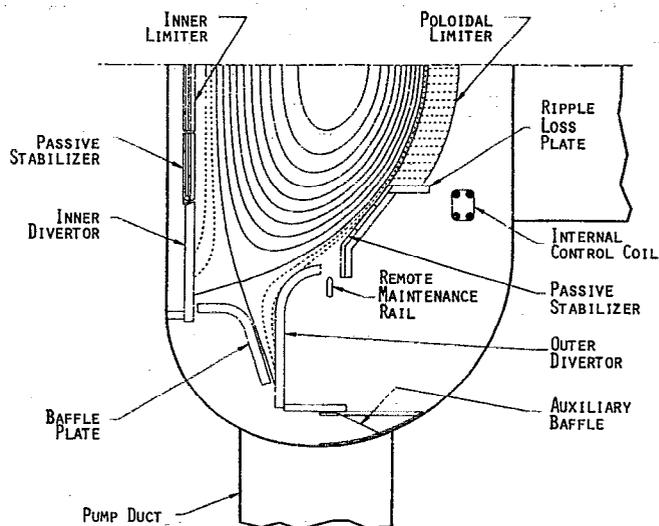
FIG. 4. Cross section of the TPX plasma magnetic surfaces below the midplane, inside (solid) and outside (dashed) the plasma's boundary separatrix. The dashed surfaces shown intersect the midplane 1 and 2 cm from the outboard boundary and at 2.5 and 5 cm from the inboard boundary. The main in-vessel components are shown and described in the text.
