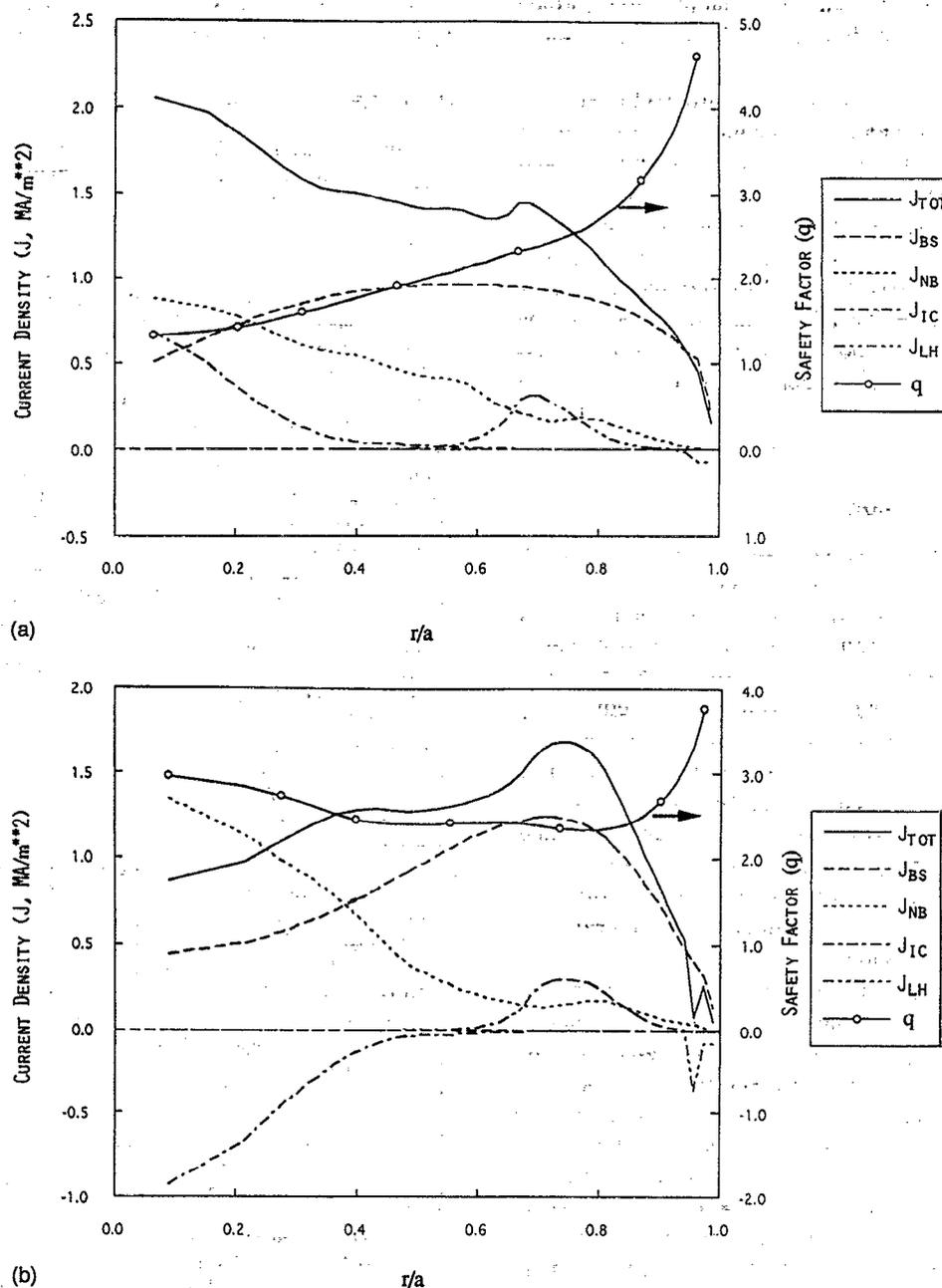
FIG. 5. Profiles of total plasma current, plasma current components, and safety factor for (a) an ARIES-I mode and (b) a reversed-shear mode.
