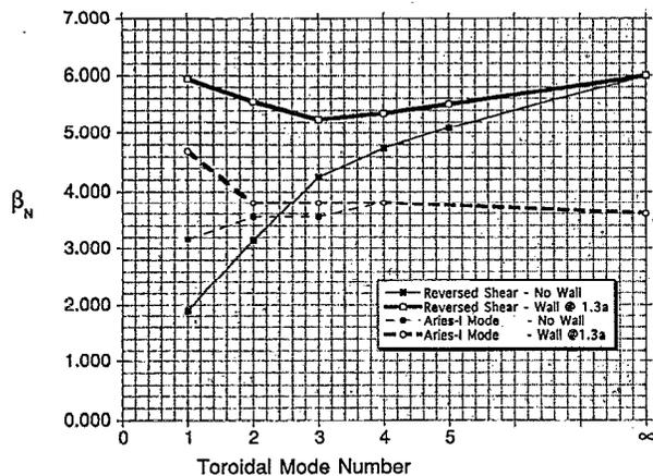
FIG. 1. Calculated ideal MHD stability for reversed shear mode ( $\beta_N=4.8$ ,  $f_{bs} = 0.93$ ) and for the ARIES-I mode ( $\beta_N=3.1$ ,  $f_{bs}=0.68$ ) with and without a conducting wall.
