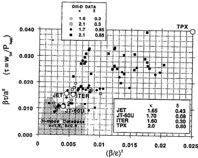
FIG. 2. Achieved values at  $\beta\tau/a^2$  and  $(\beta/\epsilon)^2$  for DIII-D VH-mode shape scan plotted against ITER H-mode database, and highest performance JET and JT-60U data. ITER and TPX target points included.
